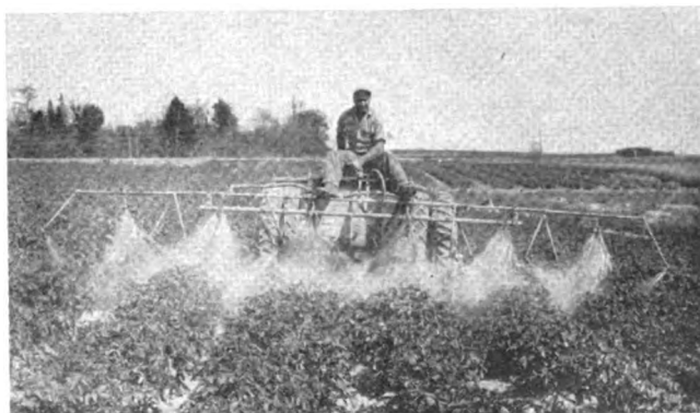
A six-row power sprayer equipped with one kind of dropped-nozzle spray boom is a frequently seen type of equipment on the farm. Exposure from some insecticides may be dangerous to the operator.
