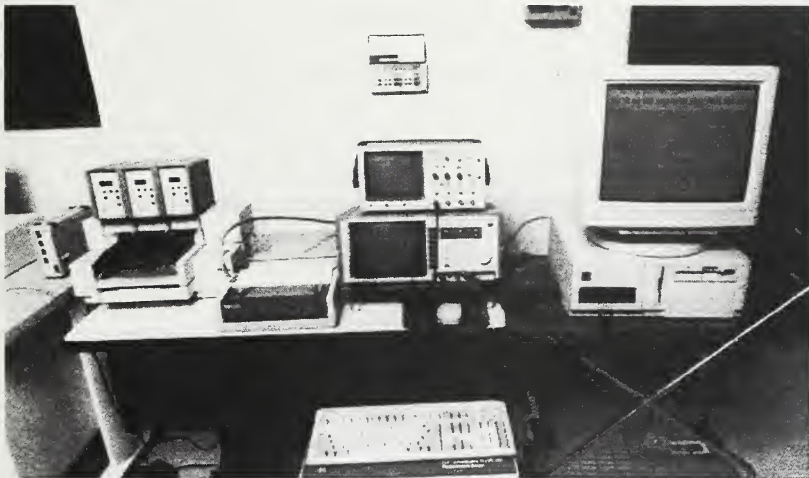
Figure D.1 MDA and high speed data acquisition computer. An oscilloscope sets on top of the MDA.
