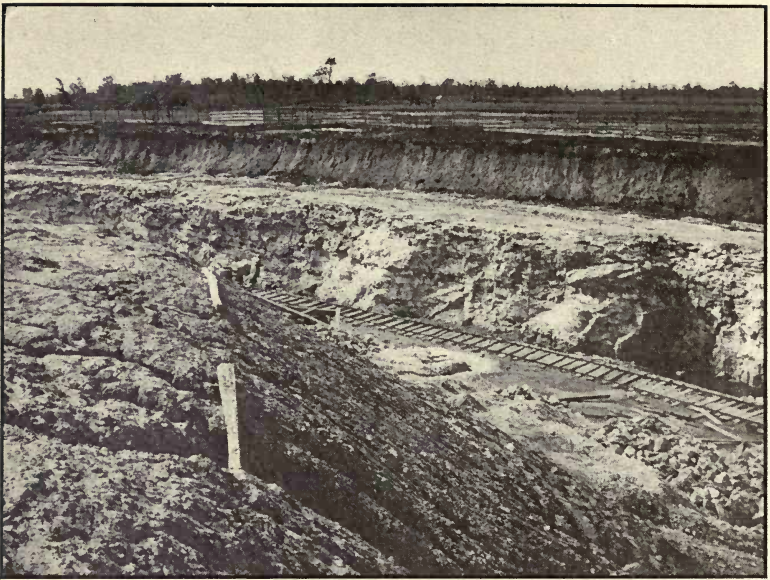
FIG. 1. — Gypsum quarry, Alabaster, Mich. Shows gypsum overlain by glacial drift. The dump in foreground is overburden removed from gypsum. Photo., A. C. Lane.
