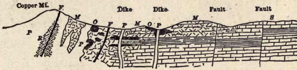
FIG. 59. — Section of Morenci district. P , porphyry; S , unaltered sediments; F , fissure veins; M , metamorphosed limestone and shale; O , contact metamorphic ores; R , disseminated chalcocite. After Lindgren, Eng. and Min. Jour. , LXXVIII: 987, 1904.
