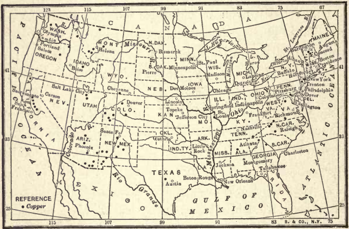
FIG. 52. — Map showing distribution of copper ores in United States. Adapted from Ransome, Min. Mag. , X: 1.
