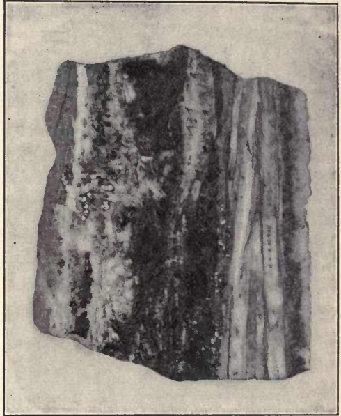
FIG. 38.—Section of vein in Enterprise mine, Rico, Colo. The right side shows later banding due to reopening of the fissure. After Ransome, U. S. Geol. Surv., 22d Ann. Rept., II : 262.
