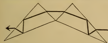
FIG. 102.—PATH OF THE RAY IN THE HERSCHEL-BROWNING SPECTROSCOPE.
