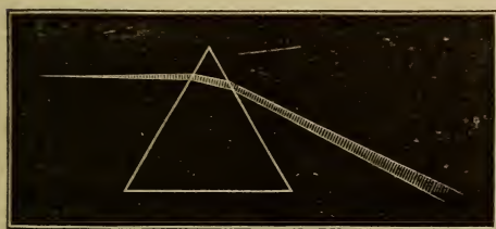
FIG. 89.—A PRISM, REFRACTING A RAY OF LIGHT.
