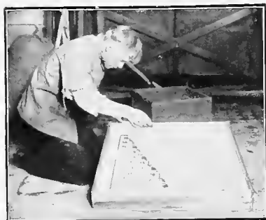
Laying on the Cover Cloth. Dip the Cover Cloth in warm water and wring it out before using.
