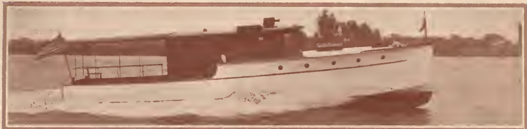
Nomabin—a 44 ft. day cruiser designed by Hacker & Fermann and built by Defoe—equipped with one 6 cyl. 200 h.p. Hall Scott Marine motor giving speed of 20 miles per hour.
