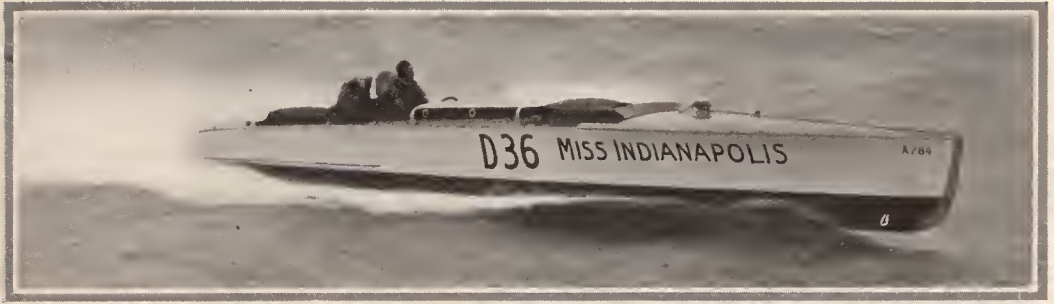
Miss Indianapolis, a Baby Gar hull, which took second place in the 150 mile Sweepstakes, averaging 47.1 miles per hour
