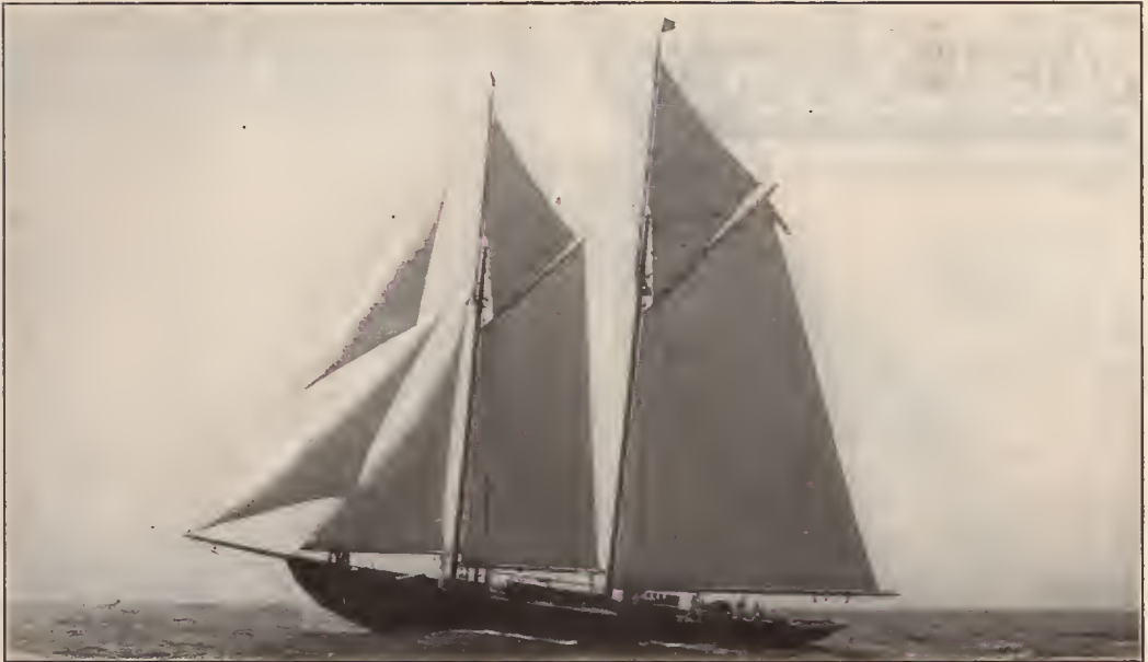
"HARDI BIAOU," 80' x 18' x 10' heavy offshore schooner, designed by John G. Alden for Dr. Henry D. Lloyd and ably powered with a Big Chief Special 75-90 H.P. Red Wing THOROBRED.
