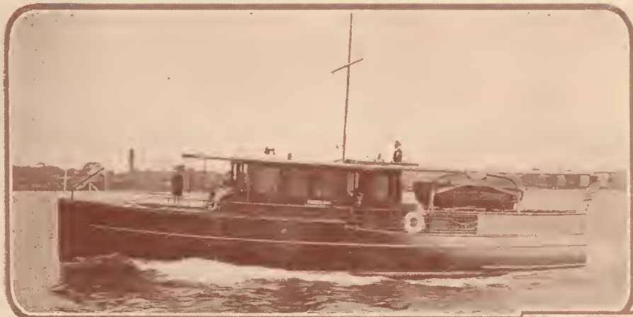
Commoore Alex McLeod's new Defoe built and Hacker Fermann designed cruiser equipped with two Sterling Sea Gulf motors (one of the H and F Standardized Fifty-fives).
