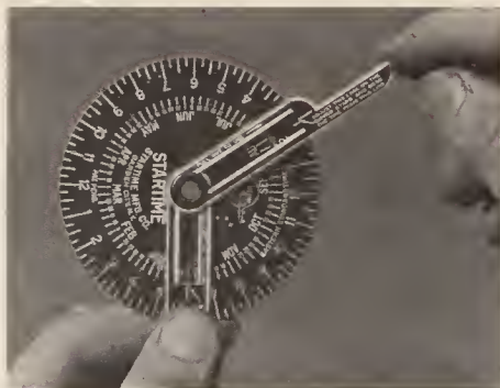
A novel star time indicator by which time can be determined closely with the pole star group
