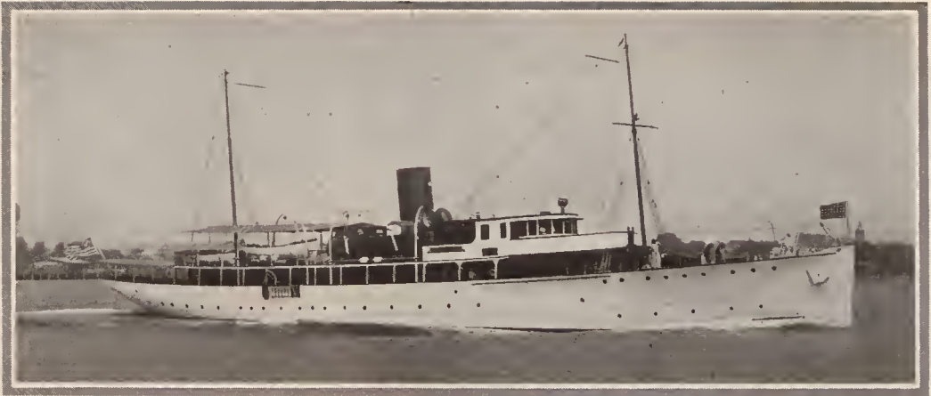
Yachtsmen have watched with interest the construction of the new 188 foot Diesel yacht Arcadia, recently completed by the Newport News Shipbuilding and Dry Dock Company from designs by Cox & Stevens. This boat is owned by Galen L. Stone of Boston, and he has stipulated a fast boat of 16 knots speed for his requirements. She is powered with two 800 h.p. Winton Diesel engines
