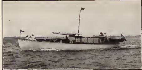
No. 415 For Sale. Herreshoff day cruiser 50 x 11 x 2' 9" draft. Four cylinder. Standard motor, speed up to 12 miles per hour. Large roomy cockpit and small cabin forward, containing two ransom berths, toilet and galley. Fine sea boat and can be purchased at a very attractive figure. Demonstration can be arranged. For further particulars regarding price, etc., consult R. M. HADDOCK, Naval Architect & Yacht Broker, 50 East 42nd Street, New York City.
