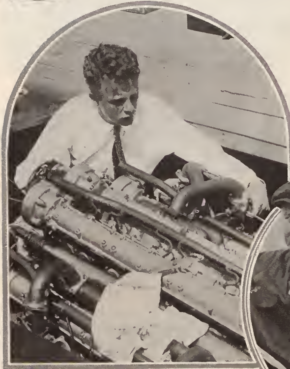
Horace E. Dodge of Detroit giving the 24 cylinder Duesenberg engine in his Gold Cup racer Impshi a final inspection before the start of the Gold Cup race
