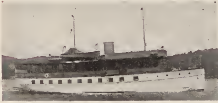
House Yacht Royono, 87' 6" x 17' x 4', just completed by the N. Y. Yacht, Launch & Engine Co. for Mr. J. B. Ford, Jr., of Detroit. Powered by two Twentieth Century 100 H.P. marine engines.
