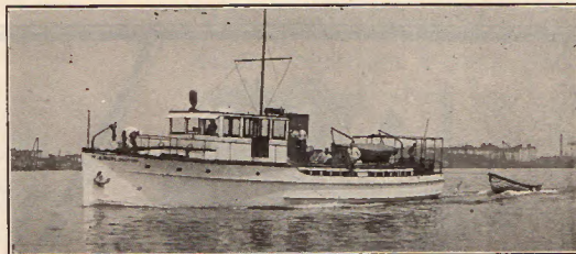
The New Jersey Fish and Game Commission Patrol Boat, H. J. Burlington, 70 feet over all, 16 feet Beam, 4 feet 9 inches Draft; powered with a 6-cylinder, direct reversing, 150 H. P. Standard Full Diesel Oil Engine.
