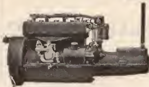
Model "R" 16-20 H.P. Bore 3-25/32", stroke 4". Price complete without reverse gear or starter, $250.00.
