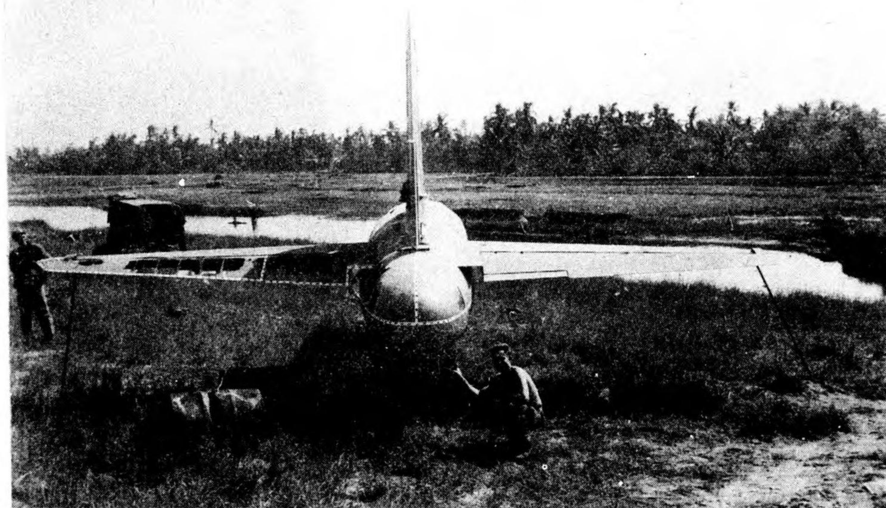
Figure 10 Rear View of Empennage and Plywood Tail Cone
