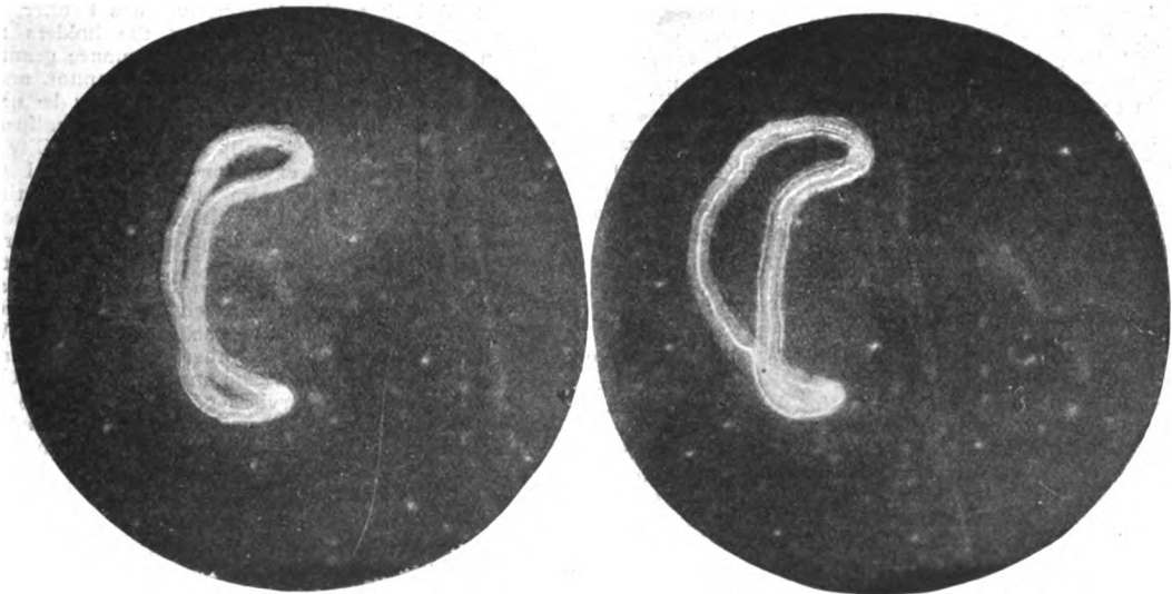
FIG. 8.—Stereoscopic view of a vibratory ring in one phase of its motion.
