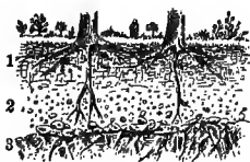
FIG. 14. — Illustrating gradual transformation of bed-rock (3) into subsoil (2) and cultivated soil (1). (After Geikie.)
