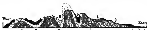
FIG. 10.—Mountain Formation. Profile through the Alleghenies. 1, Miocene; 2, Eocene; 3, Chalk; 4, New Red Sandstone; 5, Carboniferous; 6, Devonian; 7, Silurian; 8, Primary Gneiss.
