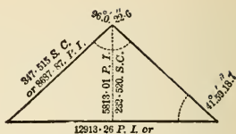
DIAGONAL VERTICAL SECTION OF GREAT PYRAMID
