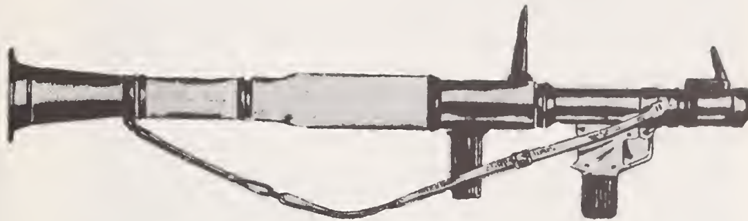
40 MM ANTI-TANK GRENADE LAUNCHER (SOVIET RPG-7), 80 MM HEAT GRENADE, EFFECTIVE RANGE 550 YDS, ARMOR PENETRATION 9.4 IN
