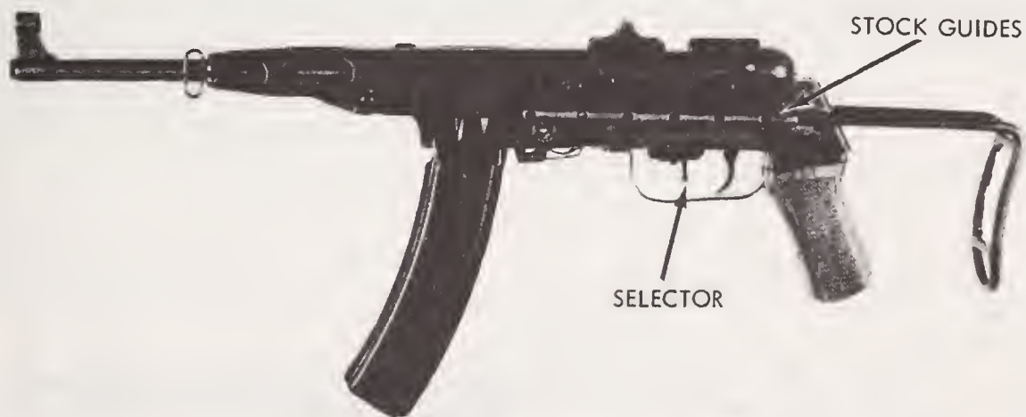
7.62 MM SUBMACHINE GUN (NORTH VIETNAMESE TYPE 50) SEMIAUTOMATIC, AUTOMATIC, 7.62X25 AMMUNITION, 900 RDS/MIN (CYCLIC) 100 RDS/MIN (PRACTICAL) EFFECTIVE RANGE 200 YDS
