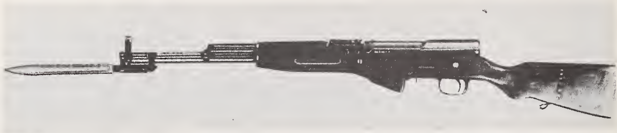
7.62 MM CARBINE (SOVIET SKS, CHICOM TYPE 56) SEMI-AUTOMATIC, M1943 AMMUNITION, 20 RDS/MIN, EFFECTIVE RANGE 440 YDS
