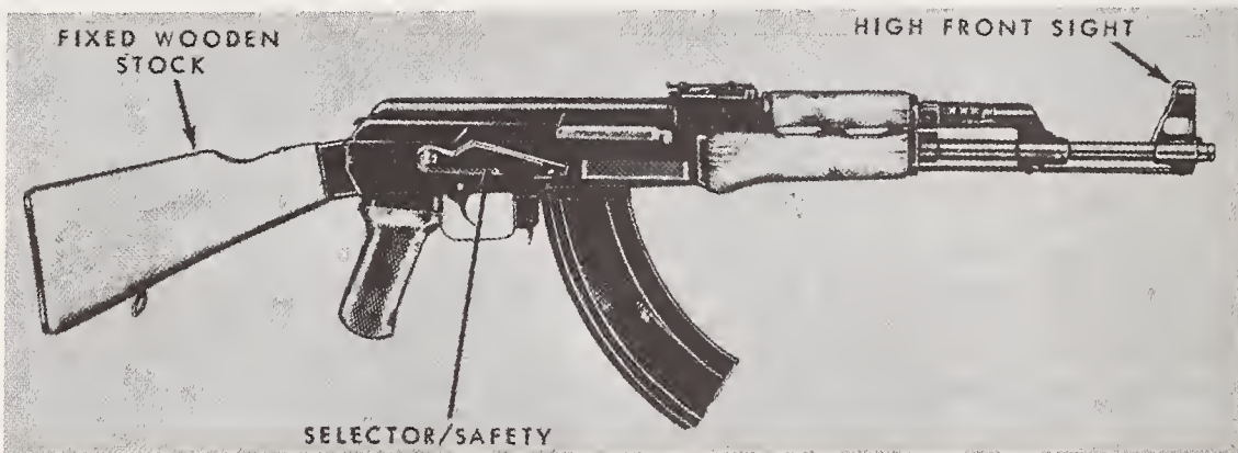
7.62 MM ASSAULT RIFLE (SOVIET AK-47, CHICOM TYPE 56) SEMIAUTOMATIC, AUTOMATIC, 7.62X 39 AMMUNITION, 600 RDS/MIN (CYCLIC) 80 RDS/MIN (PRACTICAL) EFFECTIVE RANGE 440 YDS
