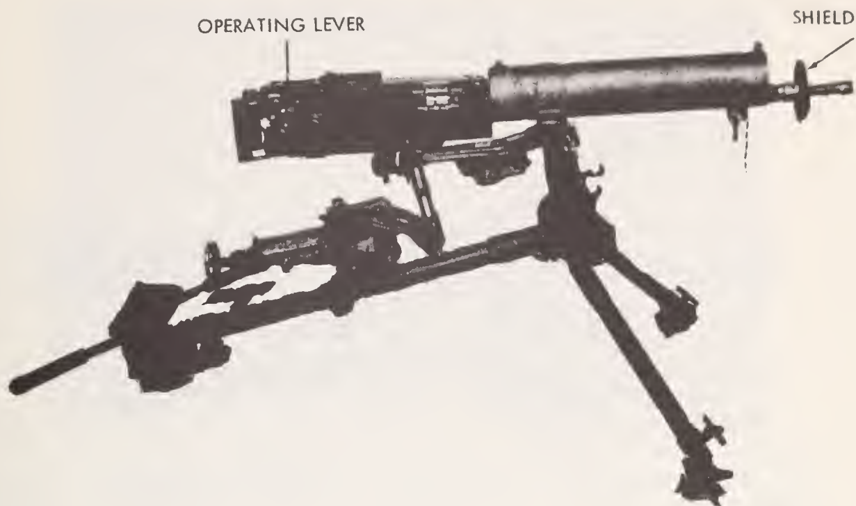
7.92 MM HEAVY MACHINEGUN (CHICOM MAXIM TYPE 24) AUTOMATIC, 7.92 MAUSER AMMUNITION, 500 - 600 RDS/ MIN (CYCLIC), 250 - 300 RDS/MIN (PRACTICAL) EFFECTIVE RANGE 1,000 METERS
