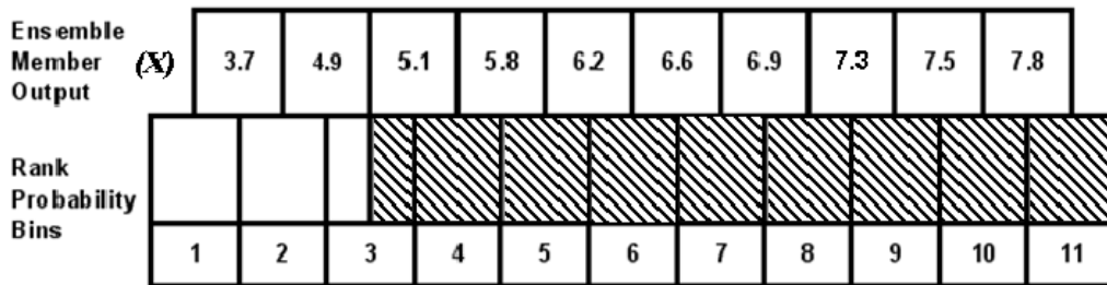
Figure 22. Uniform Ranks method. Calculating forecast probability for X \geq 5.0 using a 10-member ensemble. The probability value of 77% is represented by the hatched area [After Szczer 2008].
