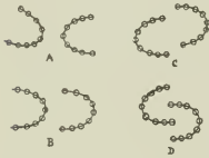
FIGURE 10.—Arrangements shown by two horseshoe-shaped aggregates. Each loop measures 30 mm. along curve; positions of magnetized needles shown by small circles. All loops in Figs. 10–16 are of similar size and construction. A , B , C , attractive pole 45 mm. above water surface; in D considerably nearer.
