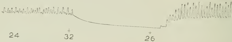
FIGURE 5.—Tracing from the ganglion-free anterior end of the heart (III). Posterior end at constant temperature of 24^{\circ} C. Temperature variations on the anterior end. Heat standstill of the muscle.
