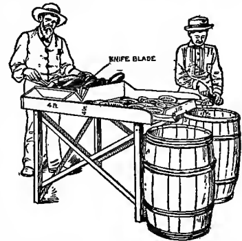
Fig. 229. Table on which cucumbers may be seeded. The fruit is emptied on the table and halved by being pushed against the set blade, and the seeds then scraped into barrels as shown.
