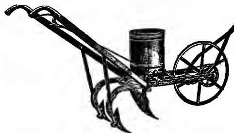
Fig. 201. One-horse combined cotton- and corn-planter.
