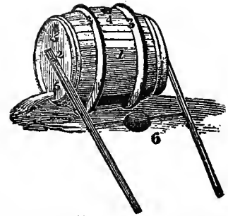
Fig. 116. "The irrigator," pictured in 1823. "This machine is calculated to water meadow-grounds, cotton and provision land, and with a boy and horse, ought to water one or two acres per day, according to the distance of the river from the field." "No. 1, The Cask; 2, The Axle; 3, Felloes; 4, Bung; 5, Plug holes at both ends; 6, Seat for the boy."
