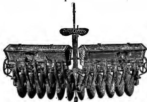
Fig. 204. Combined disk-drill and force-feed seeder.
