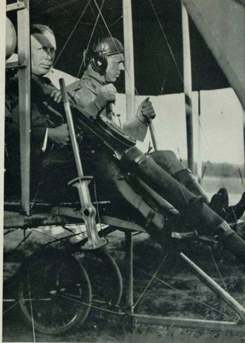
Captain C. Def. Chandler and Lieutenant Roy T. Kirtland—in Wright Type B airplanes with Lewis machine gun, June 7, 1912.—The first machine gun ever fired from airplane (Lieutenant Kirtland was pilot for test).
