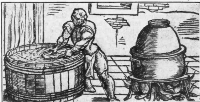
Preparing to reduce quicksilver, from Biringucci
