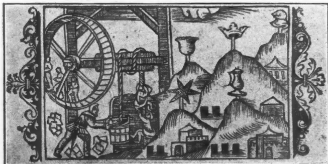
Swedish mine, sixteenth century, from Archbishop of Upsala. Note treadwheel for hoisting
