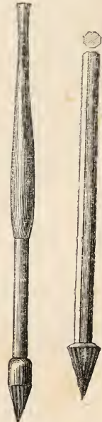
Figs. 49, 50. Drills for perforating Birds' Eggs.
