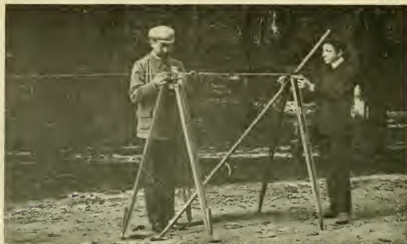
FIG. 6.—Reading the position of the end scale of the wire against a movable mark.
