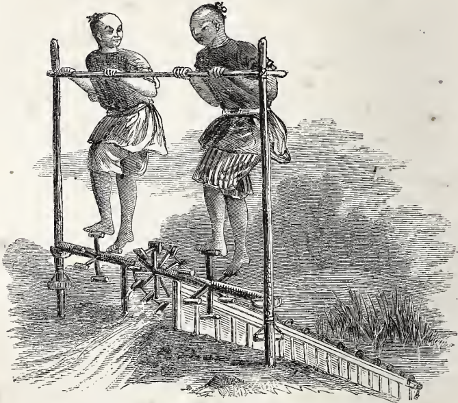
IRRIGATION BY MEANS OF AN ENDLESS CHAIN-PUMP.
