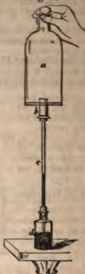
Arrangement to exhibit the Diffusive Power of Hydrogen.
