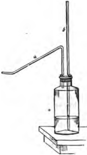
Arrangement to evolve Carbonic acid for collection over water.
