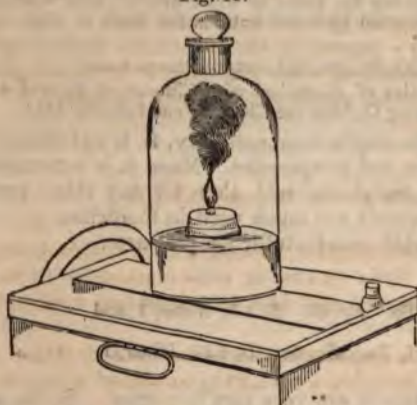
A residue of N., when Phosphorus is burned in confined Air.
