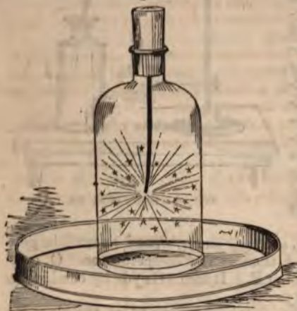
Steel burning in Oxygen.
