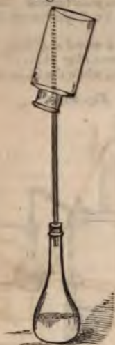
Hydrogen collected by displacement of Air.
