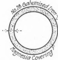
Exhaust Pipe Covering
