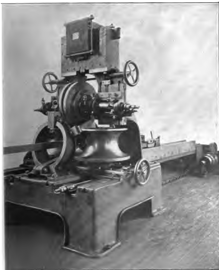
A WELDING MACHINE FOR LARGE TUBES OR SHELLS UP TO 16 INCHES IN DIAMETER, USED BY THE STANDARD WELDING COMPANY, OF CLEVELAND, OHIO.
