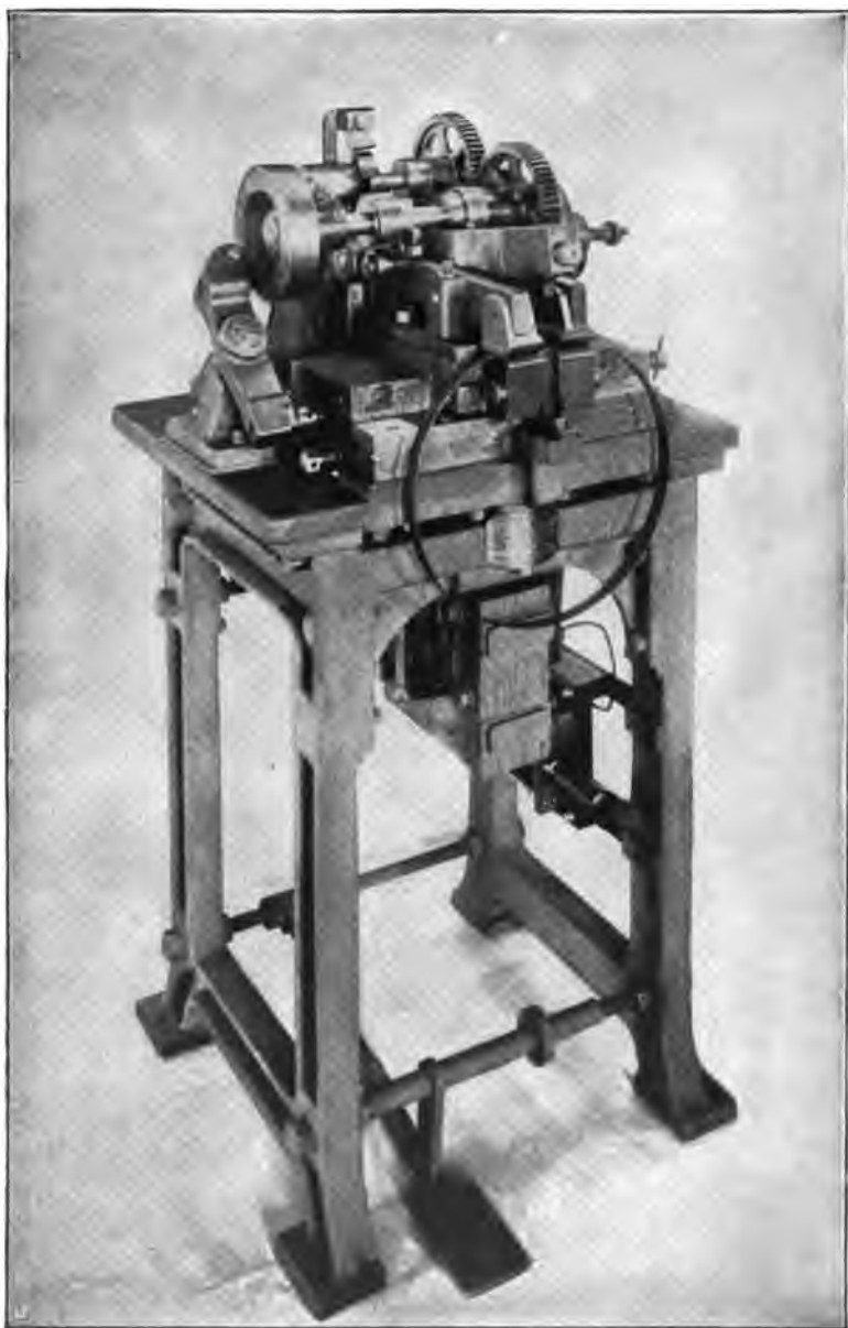
ANOTHER FORM OF HOOP OR TIRE WELDING MACHINE.
