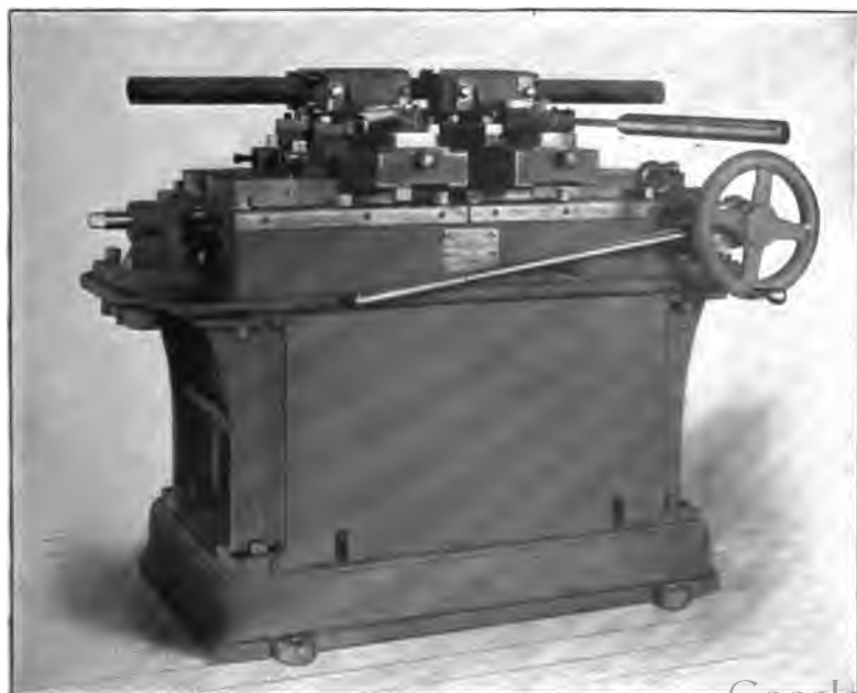
FIG. 2.—AN ELECTRIC WELDING MACHINE FOR IRON AND STEEL PIPE.
