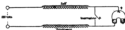
FIG. 3.—Disposition of current in Cooper-Hewitt lamp.
