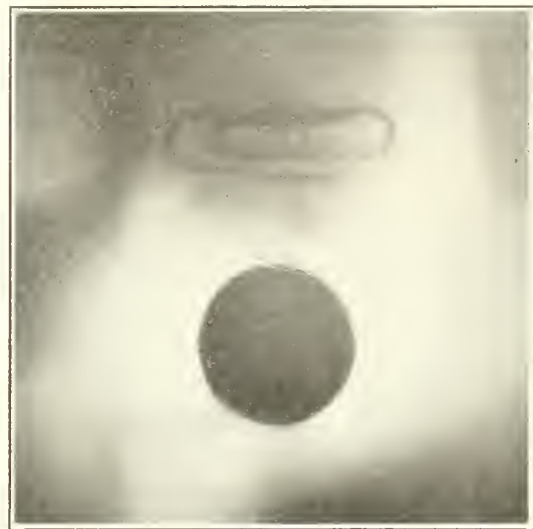
Picture No. 1—A photograph obtained by placing a piece of pitchblend on a coin and a clamp, the plate and pitchblend being bound together by two strips of adhesive plaster (see text).
