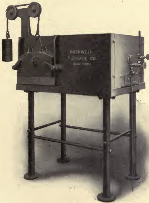
FIG. 163.—End-heating forge furnace.
