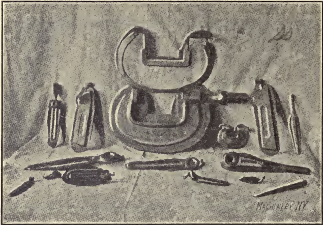
FIG. 36.—View of drop-forgings as they appear when taken from dies.
