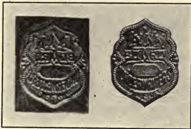
FIG. 80.—Embossed badge before and after trimming.
