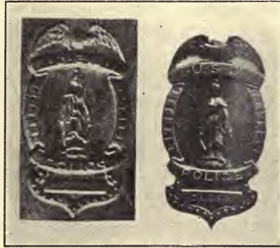
FIG. 79.—Embossed Police-shield before and after trimming.
