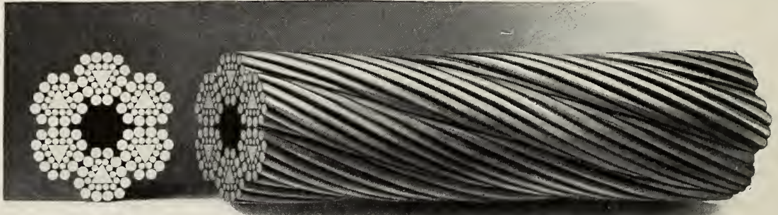
Type B—6 Strands 25 Wires—1 Hemp Core
