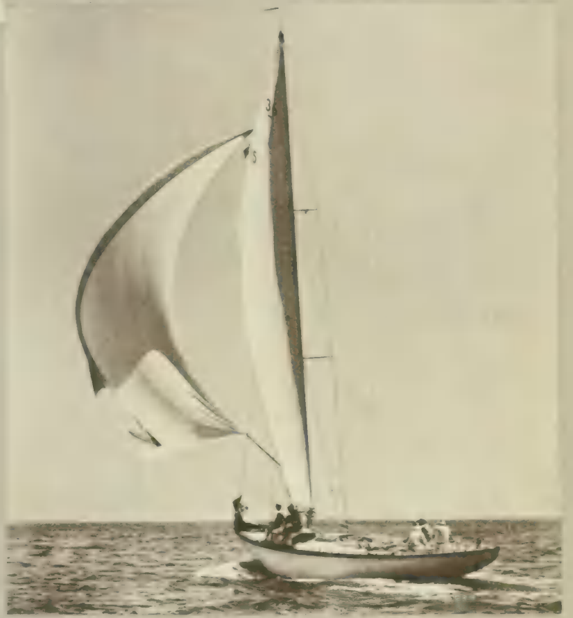
F. C. Paine's cruising cutter Gypsy is something new; no framework and made of laminated wood
