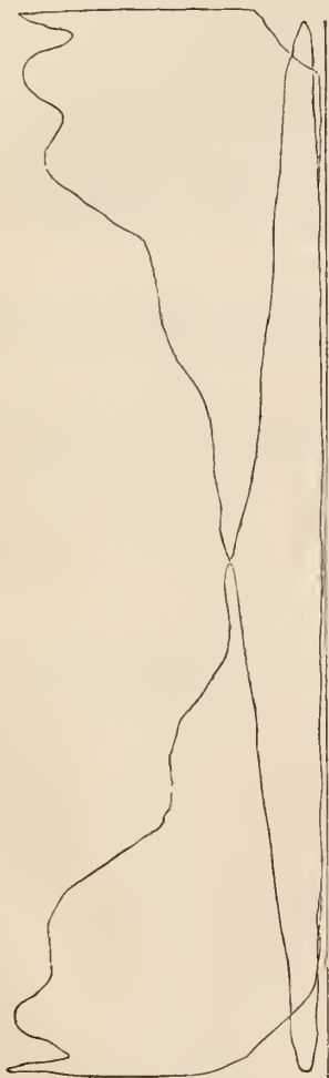
Fig. 1.—Indicator-Diagram of Messrs. Marshall, Sons, and Co.'s Portable Engine, No. 5024 (No. 2 diagram, 14 lbs. spring).
