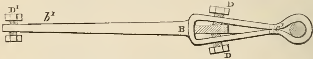
Fig. 58.—Longitudinal Section of the Beam, with the Coulter-boss and Set Screws, &c.
