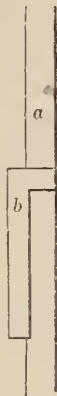
a. Beam. b. Flange of Frame resting on upper surface of Beam.
