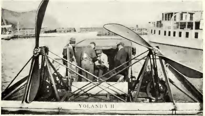
THE SEA-SLED, SHOWING THE AËRIAL PROPELLERS.
