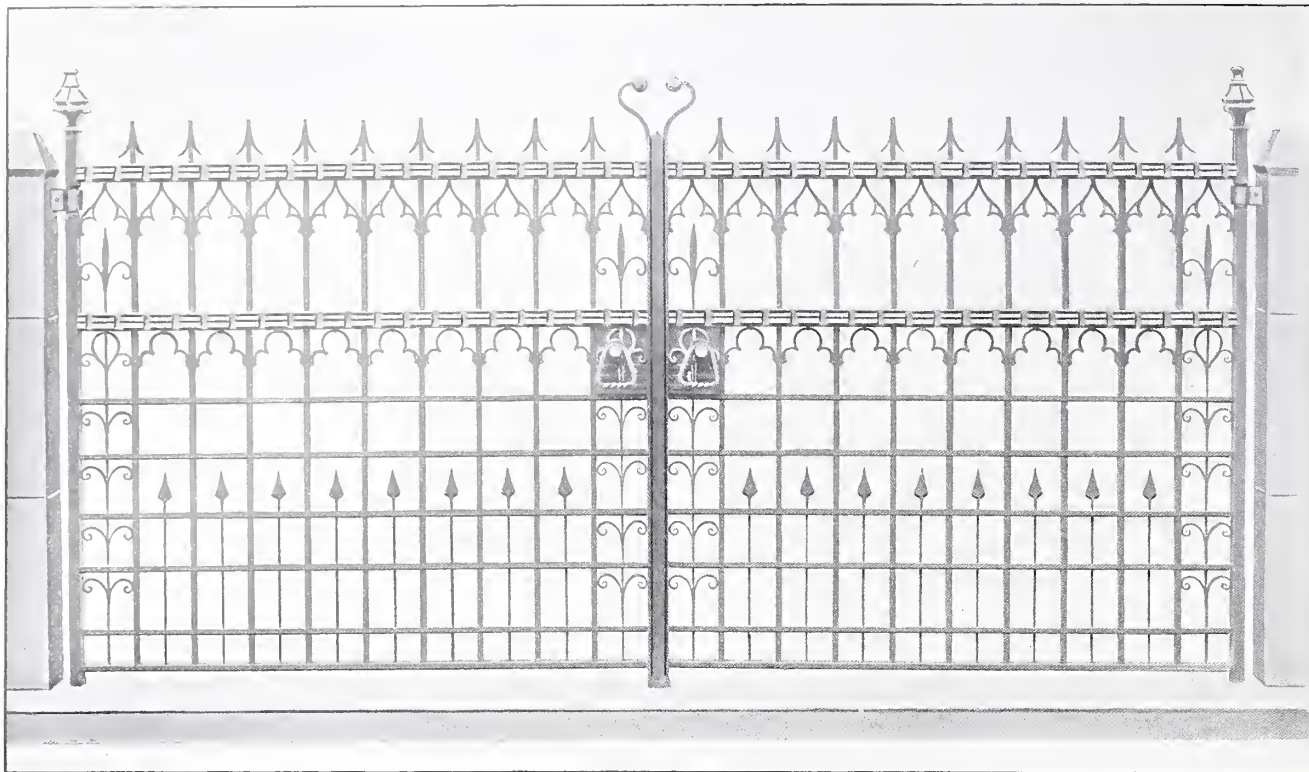
Forged Wrought-Iron Gates for Church Porch.
