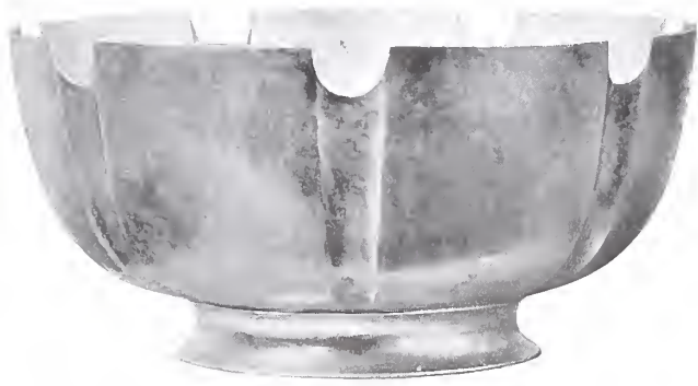
Hand-made Bowl. An example of hand-raising, leaving a thickness on the edge.
