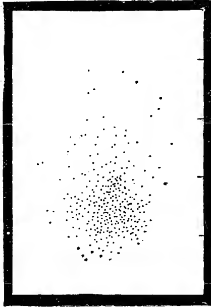
Facsimiles of patterns showing lateral deviation and stringing of the same pellets. Effects on stringing of heavy charge of powder.
