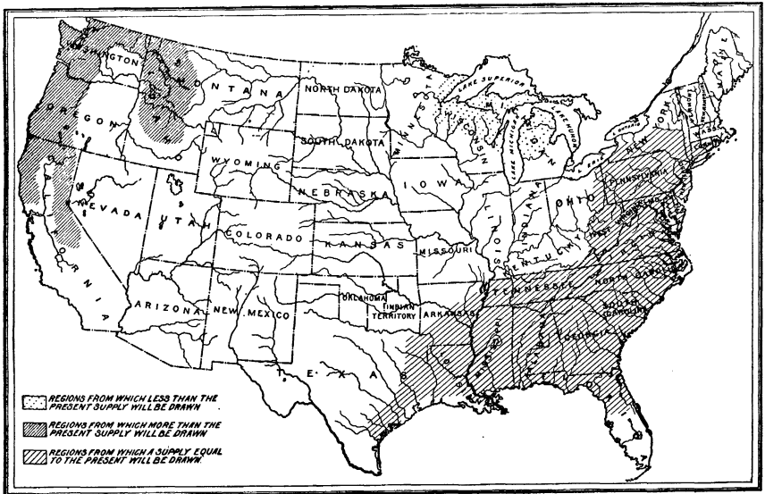
FIG. 109.—Sketch map showing main sources of future supply of pole-line construction timber.
