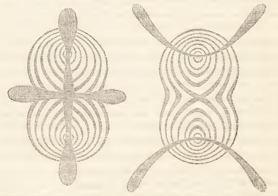
developed; and the transition of one of these forms into the other may be distinctly traced, by causing the polarizing eye-piece, whether tourmaline, pile of glass slips, or reflecting plate, to revolve. Besides nitre, there are many other crystalline bodies, such as borax, aragonite, &c. which display analogous phenomena.
