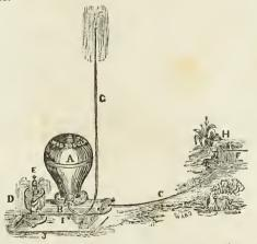
WATER RAM.—These are very useful machines for raising water wherever a fall of four or five feet can be obtained. In such cases they will raise, according to their size, from 5 to 50 gallons per minute, to a perpendicular height of 100 feet or more. These machines combine simplicity of construction with great effective power, and arc but very little liable to get out of order.
