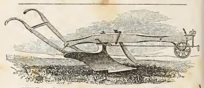
**SWARD PLOUGH**—for breaking up grass lands. These ploughs have a peculiar structure of the mould-board, or ground wrest, whereby the cohesion of the furrow slice is completely destroyed, and turned over or inverted in a light and friable condition.
