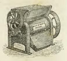
**CORN CRACKER.**—This valuable machine is used for cracking corn and cobs, previous to grinding them for provender, or for cracking the corn alone, as for hominy, or stable use. It grinds the corn and cobs to the same degree of fineness, even when the corn is damp or green, without clogging, which no other mill will do. It combines the essential requisites of compactness, durability, uniformity of work, and economy of power.
