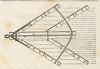
**THE GEDDES HARROW.**—The cut, it is presumed, will sufficiently explain the merits of this implement. As the draught is from the center, the uncasy struggling motion of the square harrow is got rid of, and it is consequently easier for the team; it is provided with hinges, and can be readily lifted when in motion.
