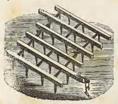
**THE SQUARE HARROW.**—The eut represents a very good form of square harrow, with folding joints, suitable for rough, heavy work.
