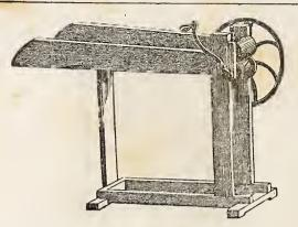
**STRAW CUTTERS.**—Of these there are a great variety; some adapted for cutting hay and straw, and others for corn stalks; and some combining the necessary requisites for doing both. They are adapted for hand use or horse power, as may be required. The latter are very powerful "machines, and will readily cut a ton of hay in an hour and a half.
