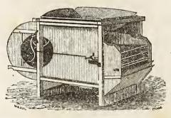
**FANNING MILL.**—Of these there are several different kinds; the best will clean at the rate of a bushel of wheat per minute, taking out all the chaff, cockle, chess, or other extraneous matter at one operation, and yet working so easily, as to only require the strength of a stout lad in turning them.
