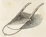
**ROAD SCRAPER.**—The best of these are now made with east iron bottoms, sides, and edges. They are very useful in road-making, leveling, ditch-making, etc., and would be found to be a useful and convenient article on every farm,
