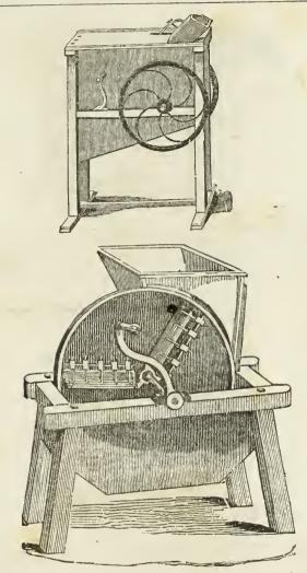
**VEGETABLE CUTTERS.**—These instruments are so improved as to cut the roots into small square pieces, and not into slices as heretofore, thus doing away with the danger of the animal choking, and also enabling it to take up its food readily and without inconvenience.
