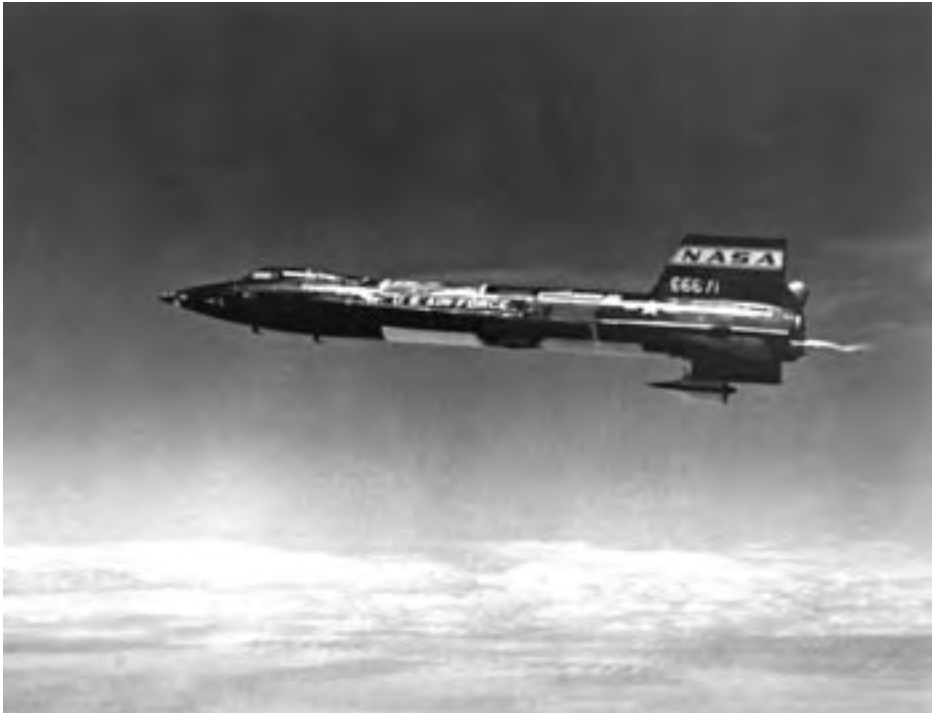
X-15 with dummy Hypersonic Research Engine mounted to the lower fin. (NASA)
