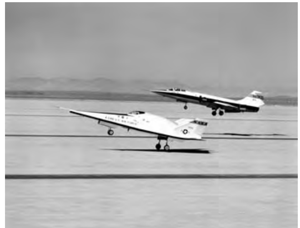
Landing a lifting body. The wingless X-24B required a particularly high angle of attack. (NASA)
