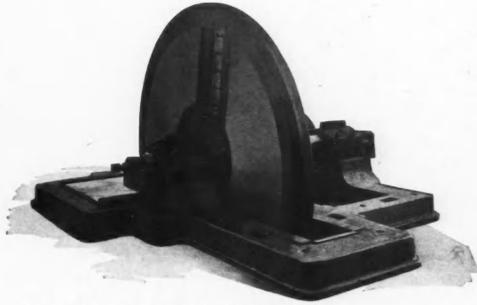
The 106-in. Improved Wolf Chipper showing disc arrangement.
