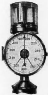
Foxboro Tachograph for recording speed of the grinder.
