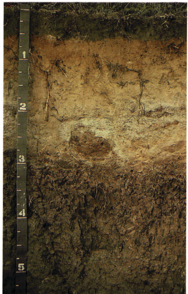
Figure 22.—Typical profile of Manistee loamy sand. The very slowly permeable clay causes a seasonally perched water table. Depth is marked in feet.
