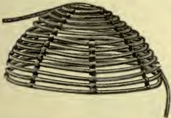
Figure 412. Water Coil for the Head.
