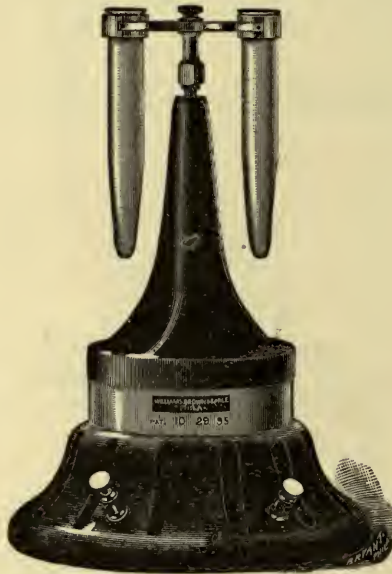
Figure 35. Purdy's Electrical Centrifuge.
