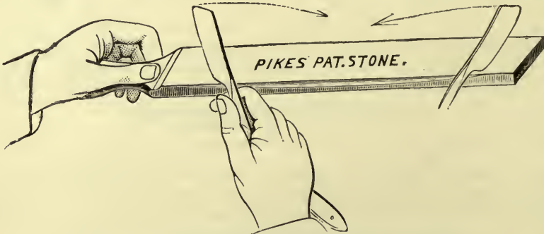
Figure 602. Showing How to Hold a Knife When Finishing the Sharpening Process.
