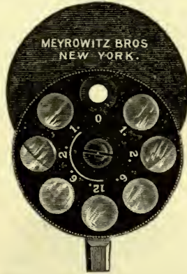
Figure 2057. Loring's 7-Lens Ophthalmoscope.
