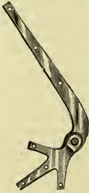
Figure 2377. Knee-Joint Irons for Amputations below the Knee.
