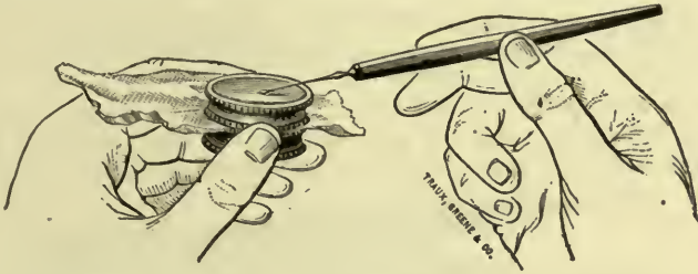
Figure 603. Test Drum for Trying Edges and Points of Instruments.
