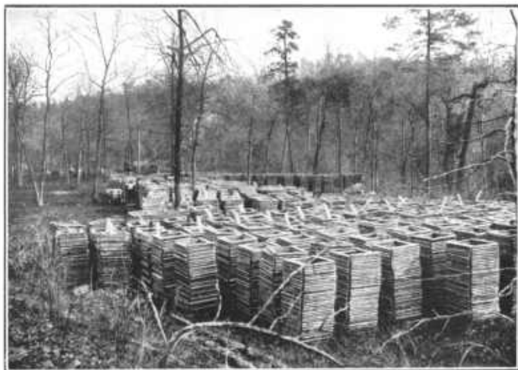
FIG. 2.—STAVES SEASONING NEAR PORTABLE MILL SET UP IN THE WOODS. WORKING UP WHITE OAK STAVE MATERIAL IN ARKANSAS.
