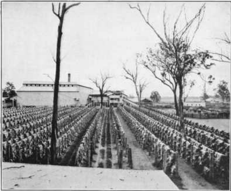
FIG. 2.—A QUEENSLAND MEAT-EXPORT WORKS, SHOWING METHOD OF DRYING SHEEPSKINS.
