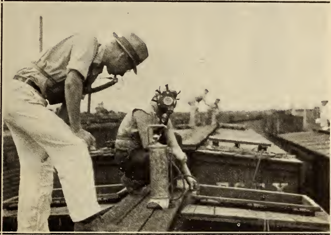
Fig. 2.—Using methyl bromide applicator in refrigerator car fumigation. Original photograph.
