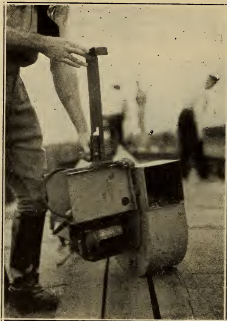
Fig. 3.—Type of blower used in fumigation of refrigerator cars with methyl bromide. Original photograph.
