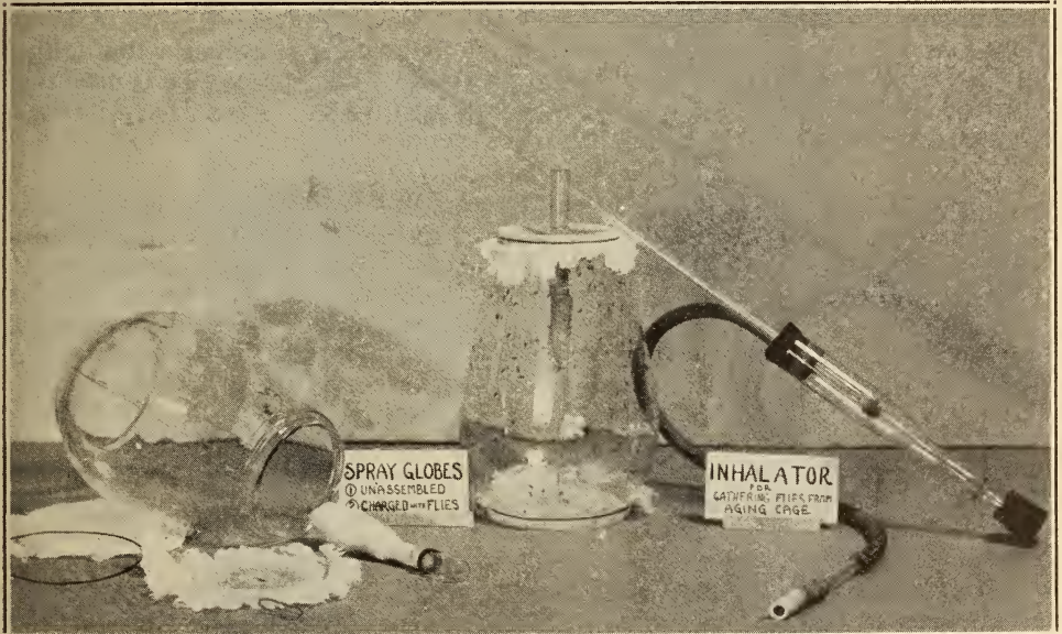
Plate 3.—Spray Globes and "Inhalator". Spray globes and apparatus for charging them. Separate items (left to right); (1) Spray globe showing parts before assembling, (2) Spray globe completely assembled and charged with flies, (3) Type of aspirator used for transferring flies.
