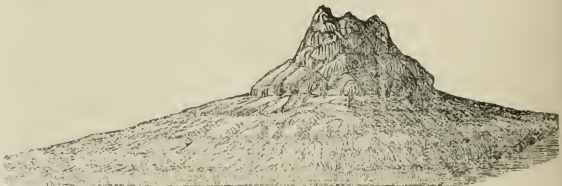
FIG. 50. PLASTER OF PARIS MODEL. Page 338. Contrived to imitate the formation of terraces of loose materials on a slope, under water, near the surface, while the water-line is gradually sinking.
