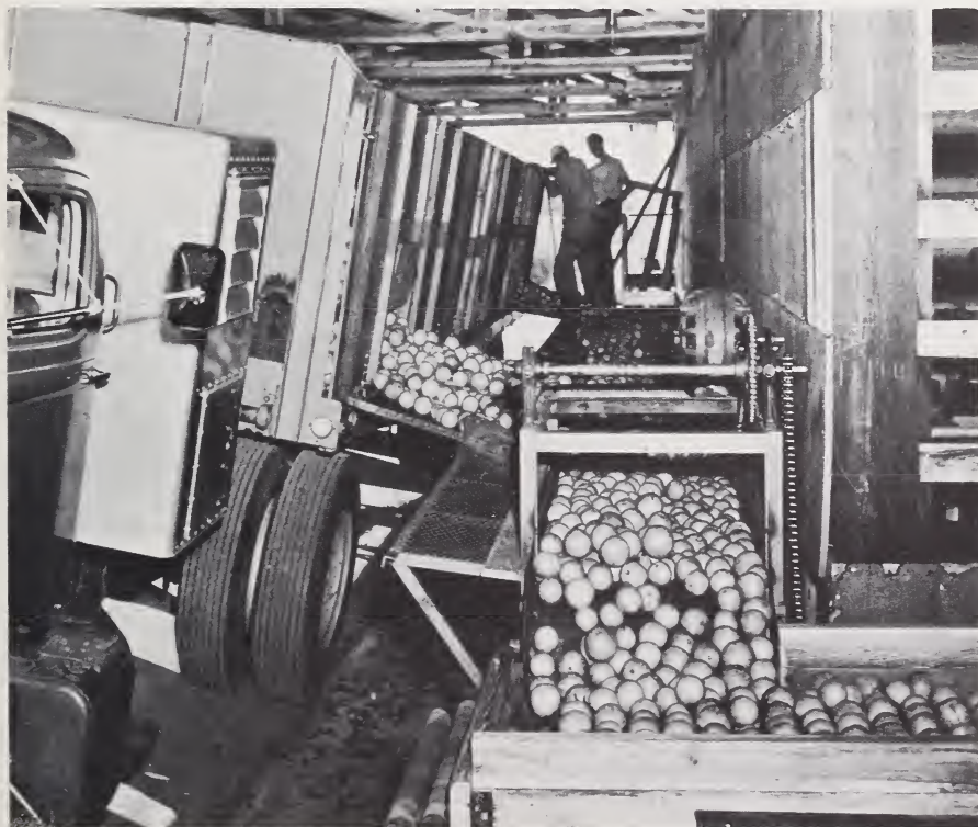
In 1948, the Fruit and Vegetable Section helped test pilot-scale equipment for developing a practical method of handling citrus fruit in bulk from grove to packinghouse. Findings from this study in Florida and California led to adoption of such equipment in citrus producing States.
