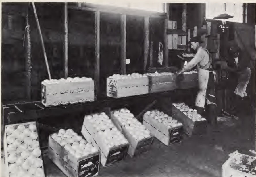
Packing oranges in Covina, Calif., in 1896. Individual wrapping of fruit and hand nailing of boxes were the usual methods of the day.
