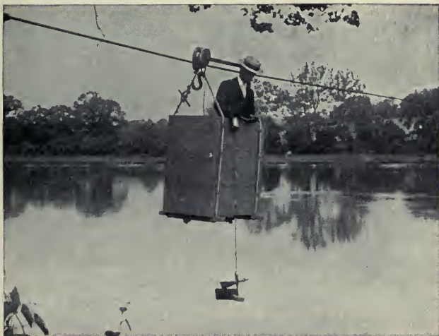
B. METHOD OF USING ELECTRIC CURRENT METER FROM SUSPENDED CAR.
