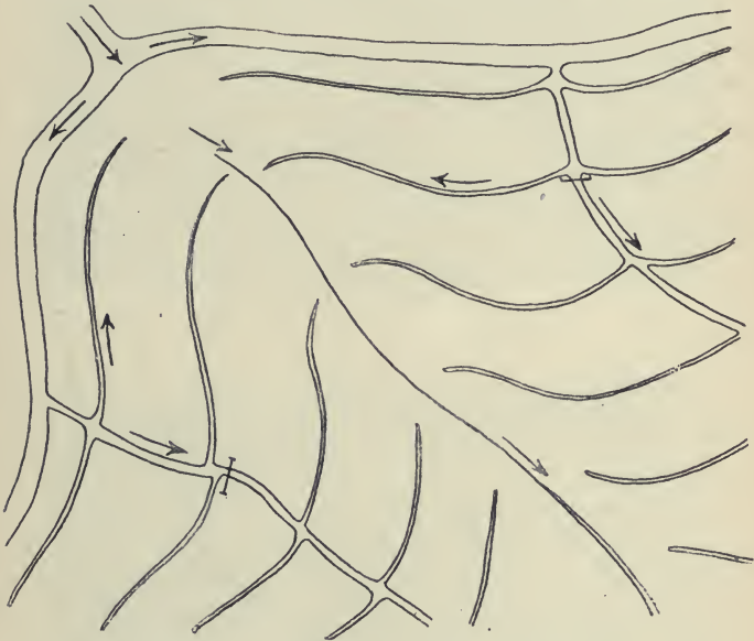
FIG. 63.— Plan of distributing water on rolling lands.
