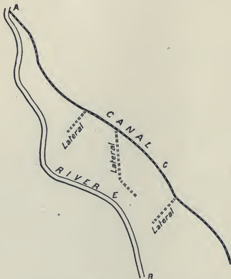
FIG. 22. — Diagram showing method of diverting a canal from a river.
