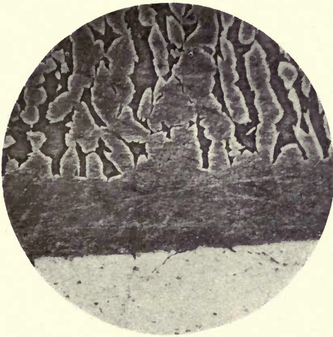
B. Diffusion of zinc into copper. \times 30 .
