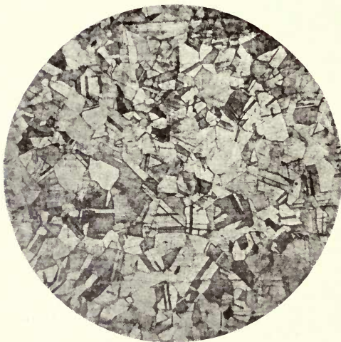
B. Brass (Cu 70, Zn 30%) annealed. \times 86 .
