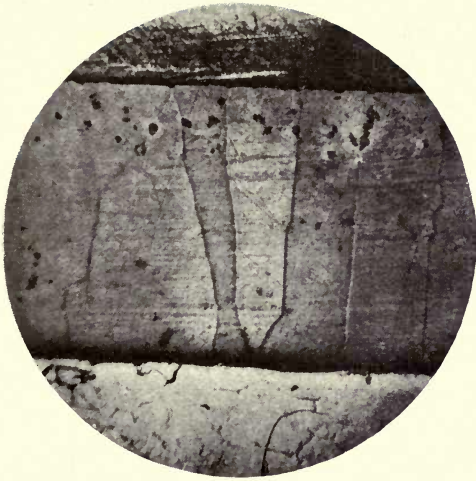
A. Diffusion of zinc into copper. \times 30 .
