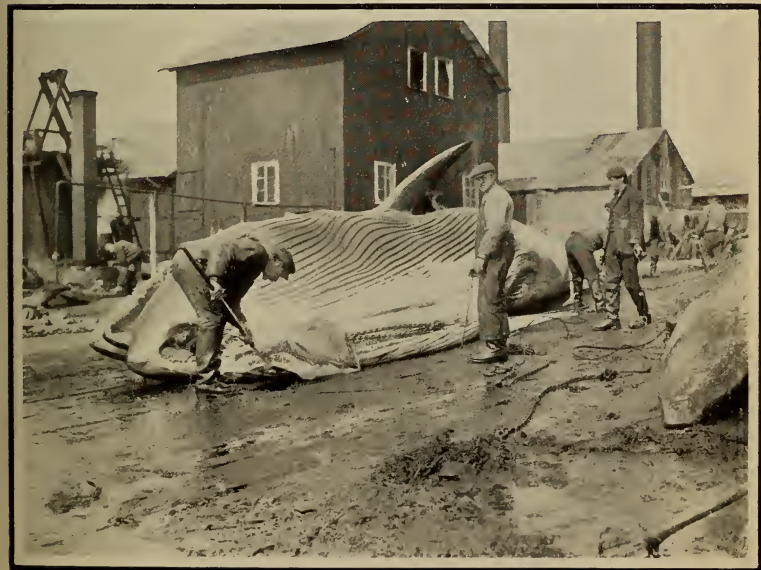
A FINNER WHALE BEING CUT UP Commencing to cut strips of the blubber with a flensing knife. The blubber is being pulled away as the man cuts by a chain and steam winch.
