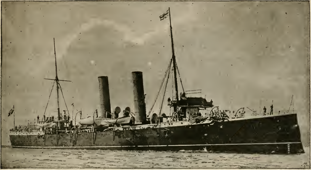
H.M.S. "LATONA," ONE OF THE SWIFTEST SHIPS IN THE ROYAL NAVY, 3,400 TONS, 9,000 HORSE-POWER.
