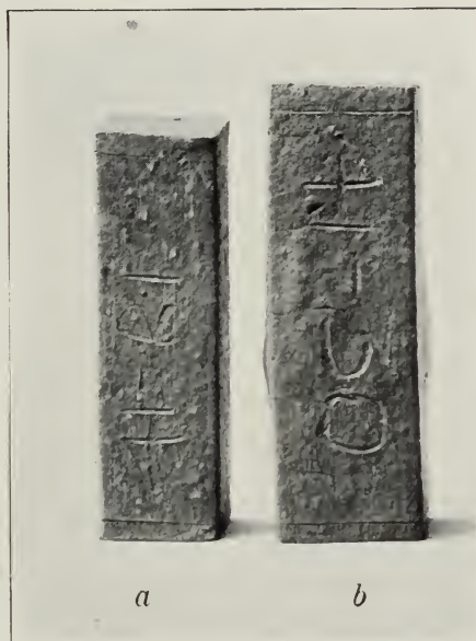
FIG. 3.—Briquets showing proper burning and overfiring.
