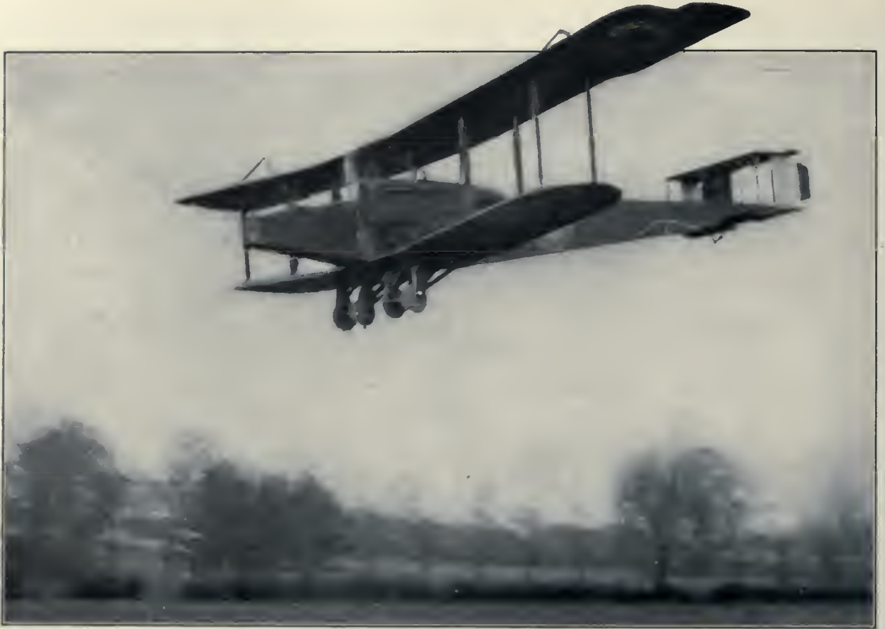
The Twin-Motored Handley Page Bombing Biplane. A Handley Page has flown from London to Asia Minor, with stops, and dropped bombs on Constantinople. It carried seven men, spare motors and supplies. Larger Handley Pages can fly across the Atlantic and bomb the German bases and munition plants.
