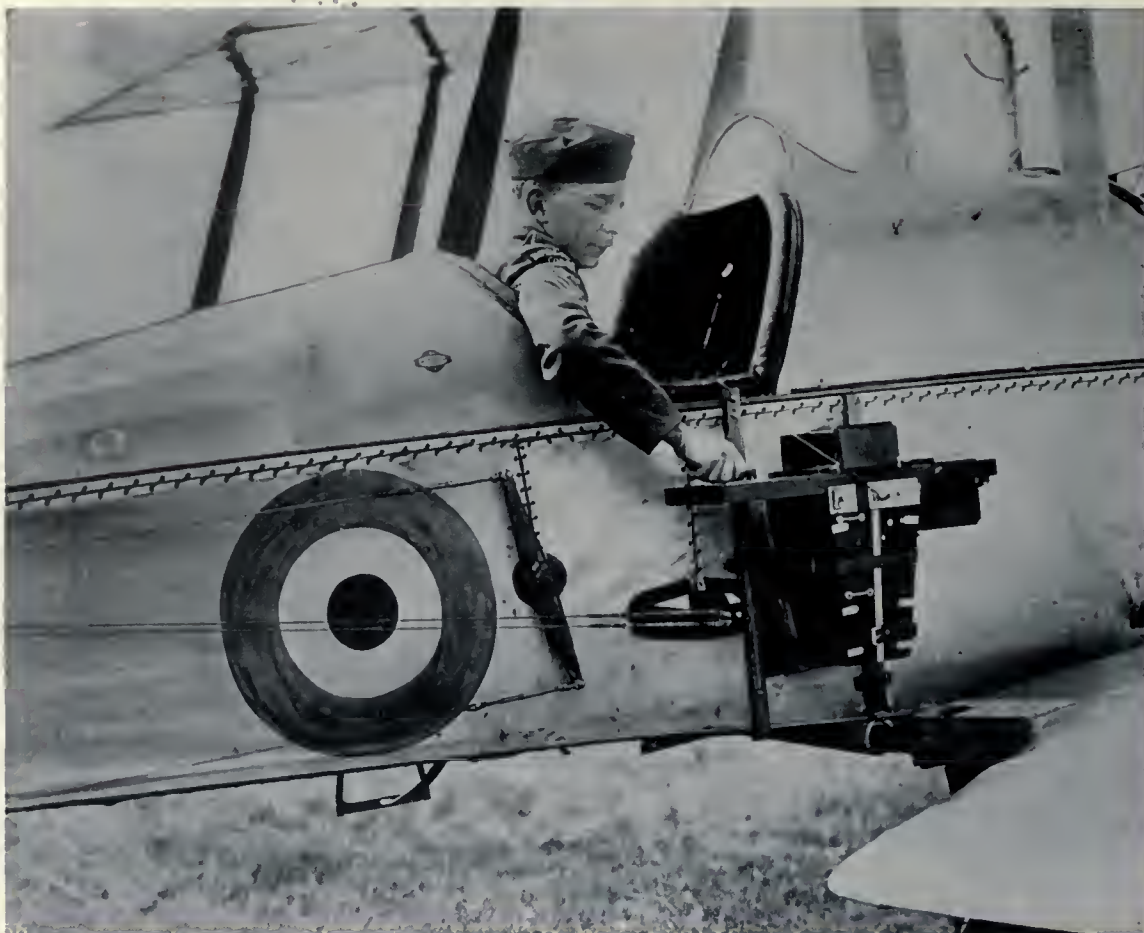
Camera mounted on a British B. E. biplane, Major Campbell in the pilot seat, demonstrating it. (Photo Bureau of Public Information.)
