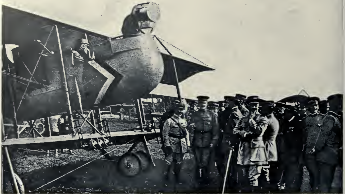
French aeroplane for night operations showing the searchlight on the machine and small lights under the bottom wing. General Pershing is visiting French aviation camp.
