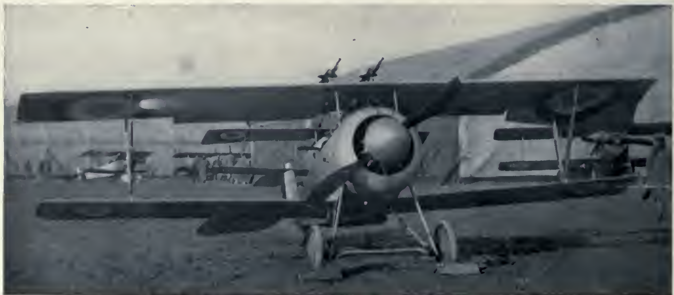
The 1917 type Nieuport avion de chasse, equipped with two Lewis guns shooting over the planes, and a Vickers gun to shoot through the propeller. In the rear can be seen a "Spad" and several Nieuports.
