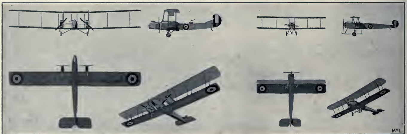
Avro (A. V. Roe & Co., Ltd.) (British). The Avro machines have an equal upper and lower wing-span. In the twin motored machine the engines are carried on the lower plane, with exhaust stacks running up over the upper plane. Vertical engines are used. A wheel is located beneath each of the two engines. The two-seater Avro has highly staggered wings and a slight dihedral. The landing gear is characteristic; the long central skid is located between the wheels, supporting V struts at either end. The rudder is of the balanced "comma" type. There is no vertical fin. A rotary engine is used.
