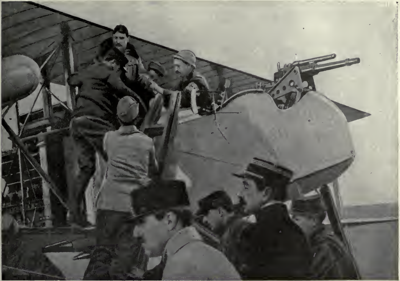
The French Bréguet-Michelin bombing biplane equipped with a 220 Peugeot motor and two guns
