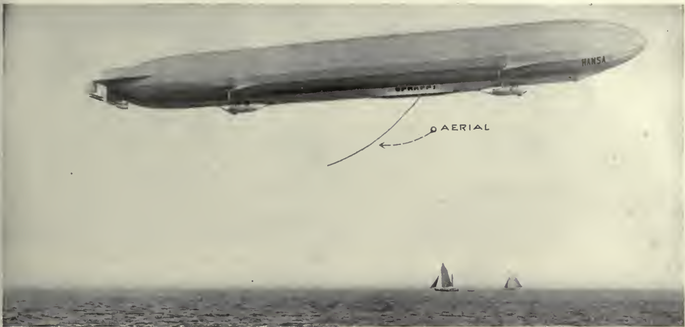
Photograph of Zeppelin showing the aerial hanging down.
