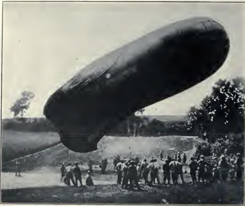
One of hundreds of Kite Balloons, which serve as the eyes of the artillery on all the fronts, being towed by its mooring-rope to its anchorage. There is a Kite Balloon for every heavy gun. An account of how Kite Balloons are operated for artillery was given in "Flying" for December.
