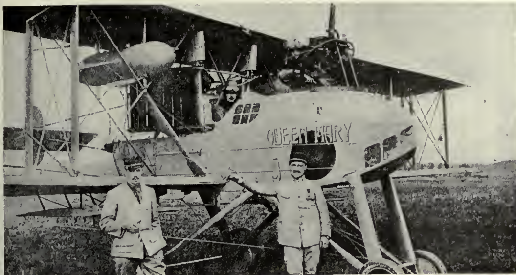
The French Bréguet Michelin warplane, equipped with one 220 horse-power Peugeot motor. This machine is used extensively for bombing.
