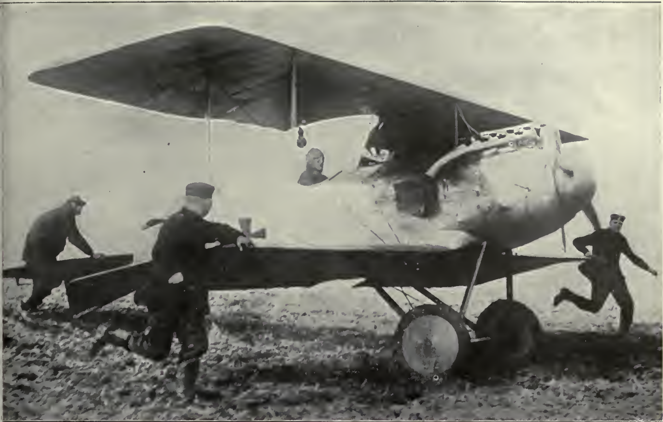
The German "Spad," the 175 h.p. Mercedes motored "Albatros" combat biplane. It carries two Maxim guns which are synchronized to shoot through the propeller.
