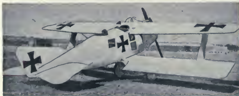
The German “Roland” two seater, so built that the pilot sees over the upper plane and has but a single strut, like the “wireless” Curtiss of 1916. It is equipped with a 150 h.p. Benz motor.
