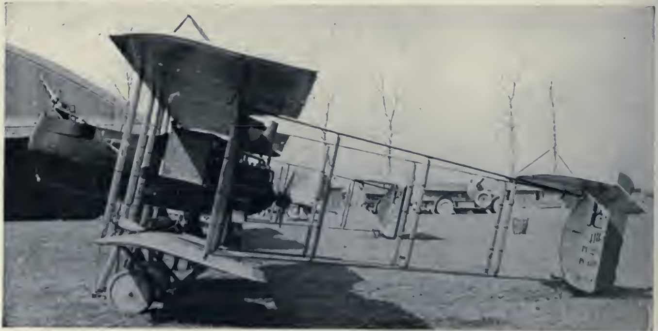
The French Farman machine equipped with a Dietrich motor, used extensively for bombing.
