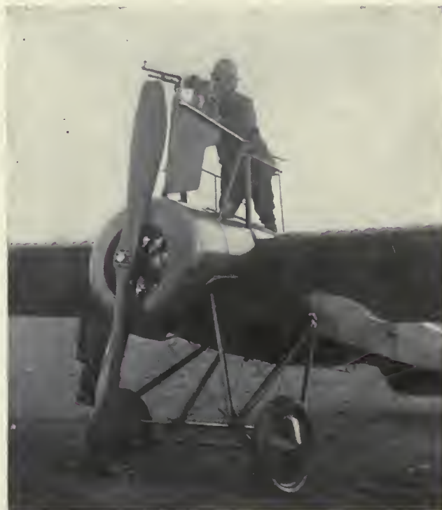
How they tried to shoot over the propeller up to 1915, before the method of synchronizing the gun with the propeller to permit shooting through it was found, a French improvement.
