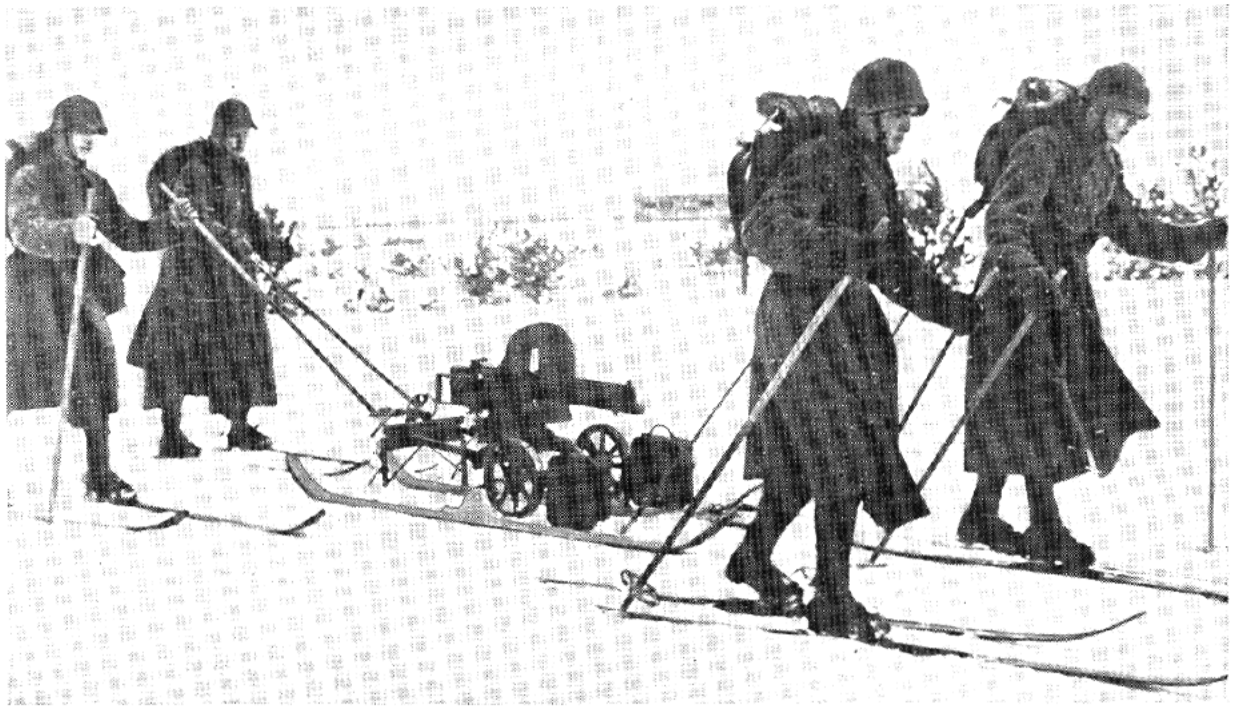
Figure 1-10. The Russian Maxim Machine Gun on ski transport, as used in the U. S. S. R. invasions of Finland in the nineteen forties.
