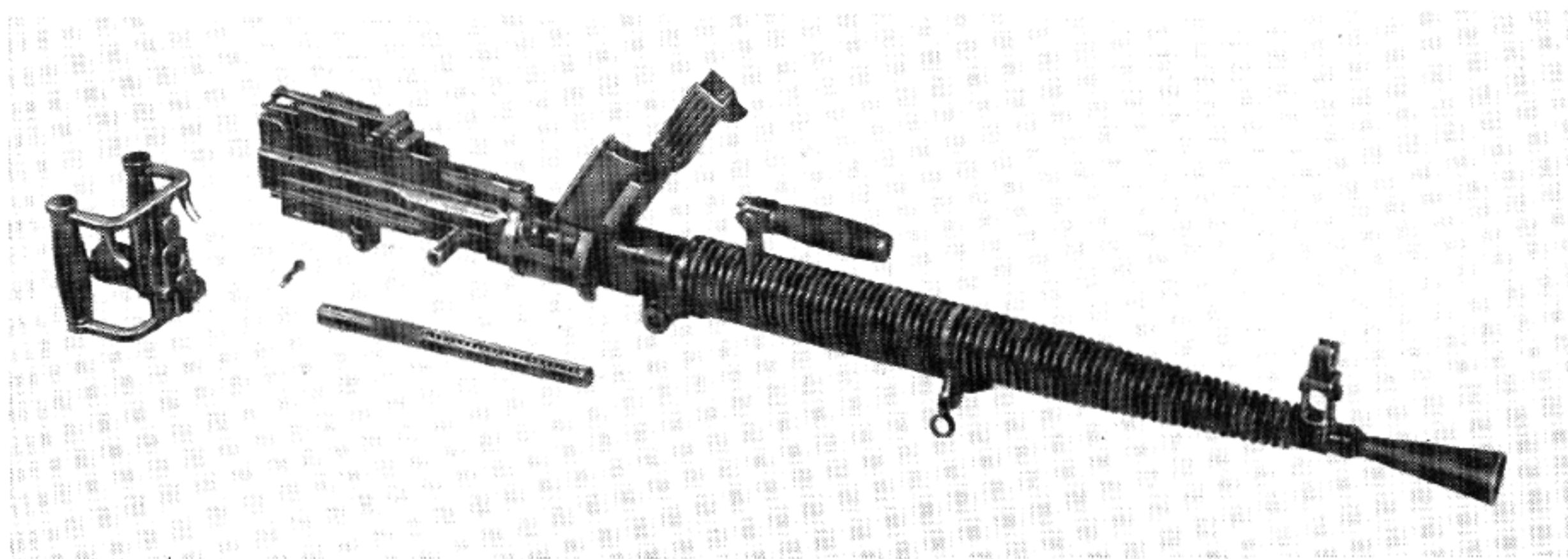
Figure 3-20. Stripping the DS: back plate group and housing removed.
