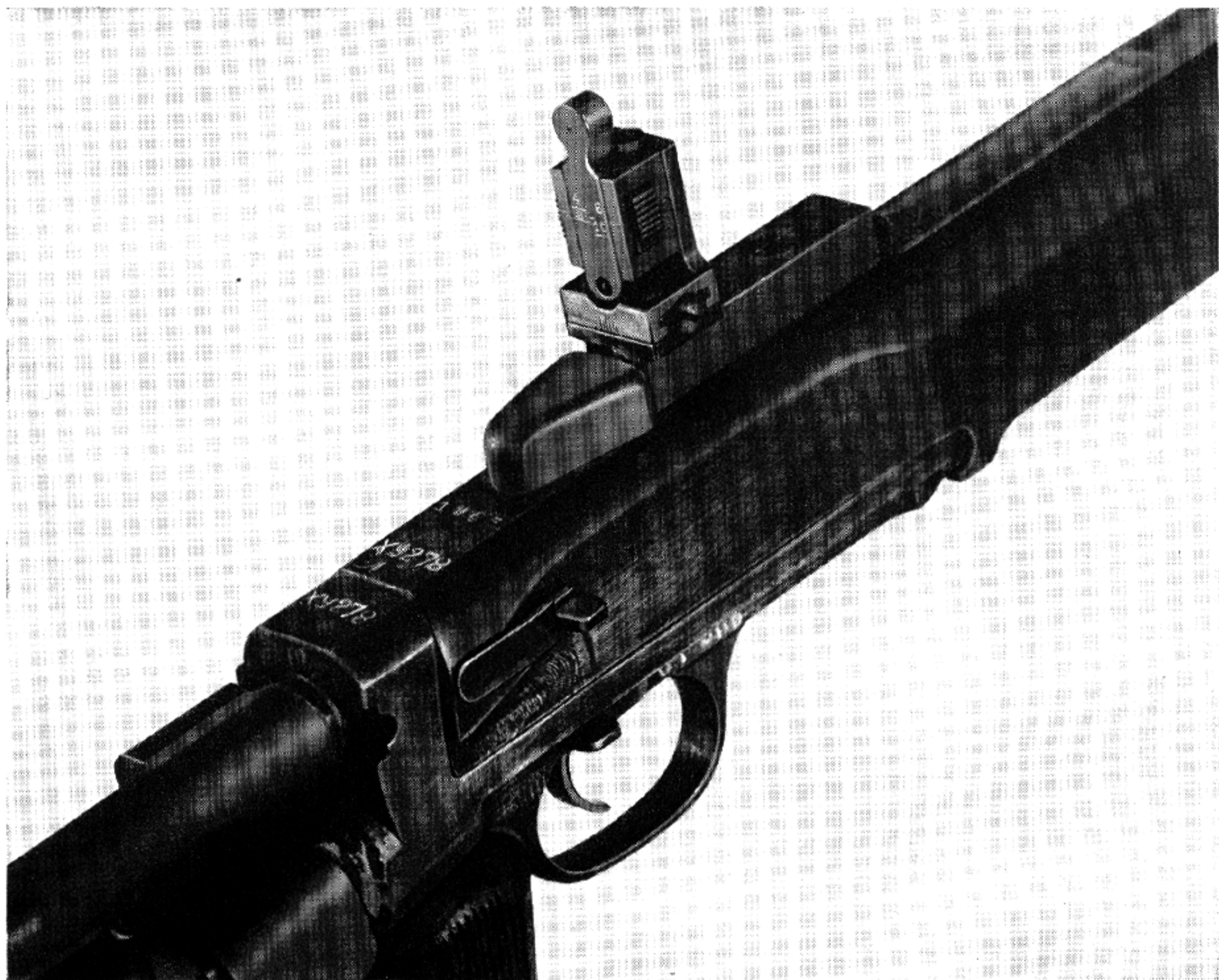
Figure 3-15. Close-up of the receiver of the DTM. The housing for the driving spring protrudes to the rear. The year of manufacture appears just behind the rear sight.
