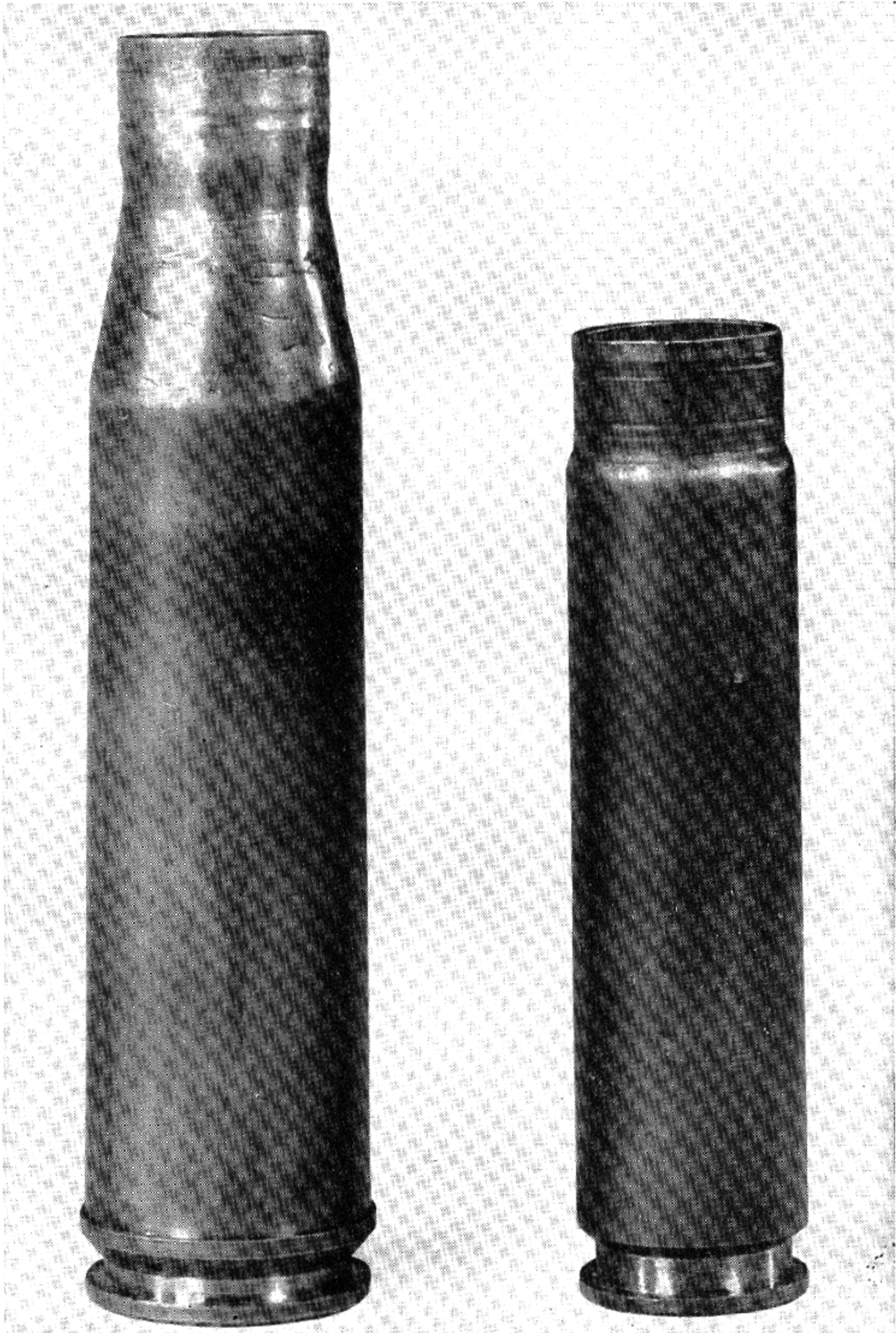
Figure 9-17. Comparison of Soviet 23-mm cartridge cases, both of which can use the same projectiles. Left case, old, for VYa type, right, new, for NS cannon.
