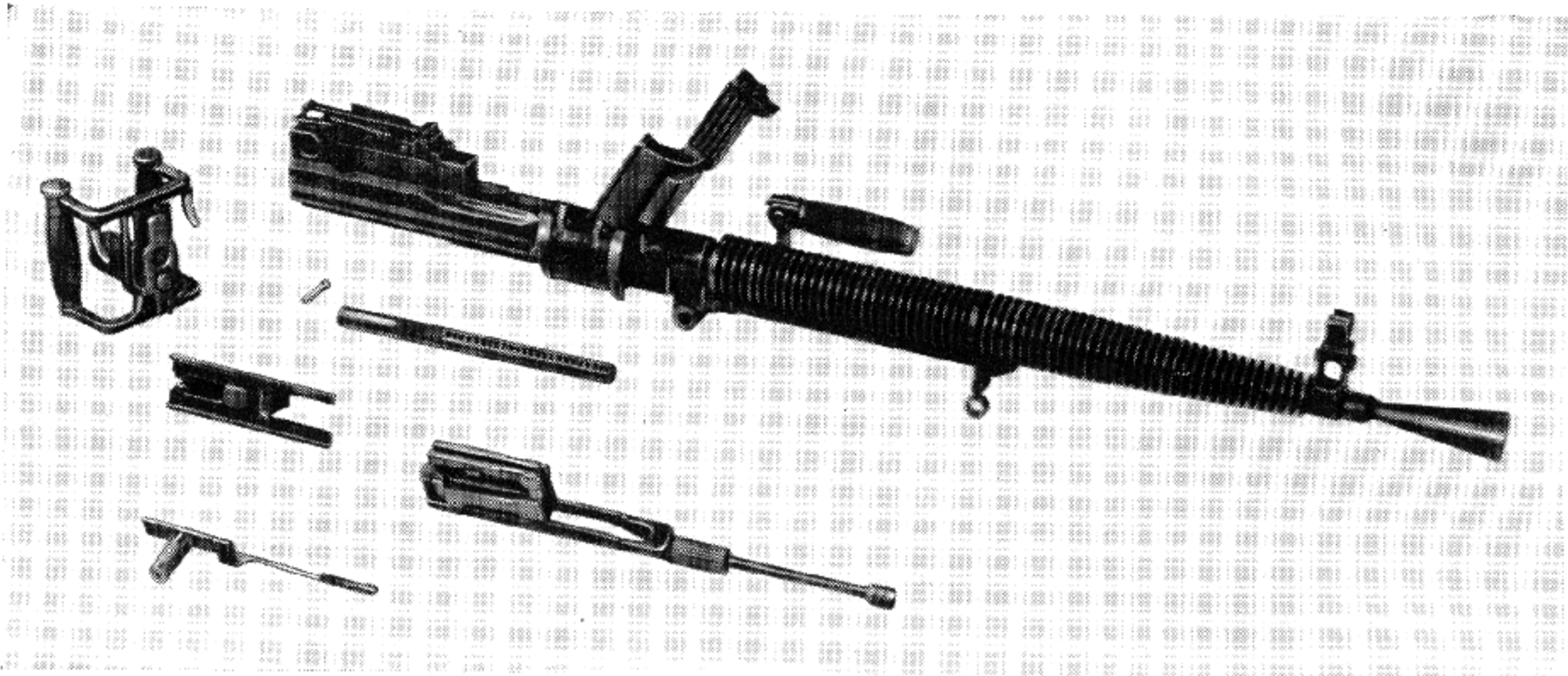
Figure 3-22. Stripping the DS, continued: operating slide and belt group have been removed together. The next step is the removal of the handle from its guideway.
