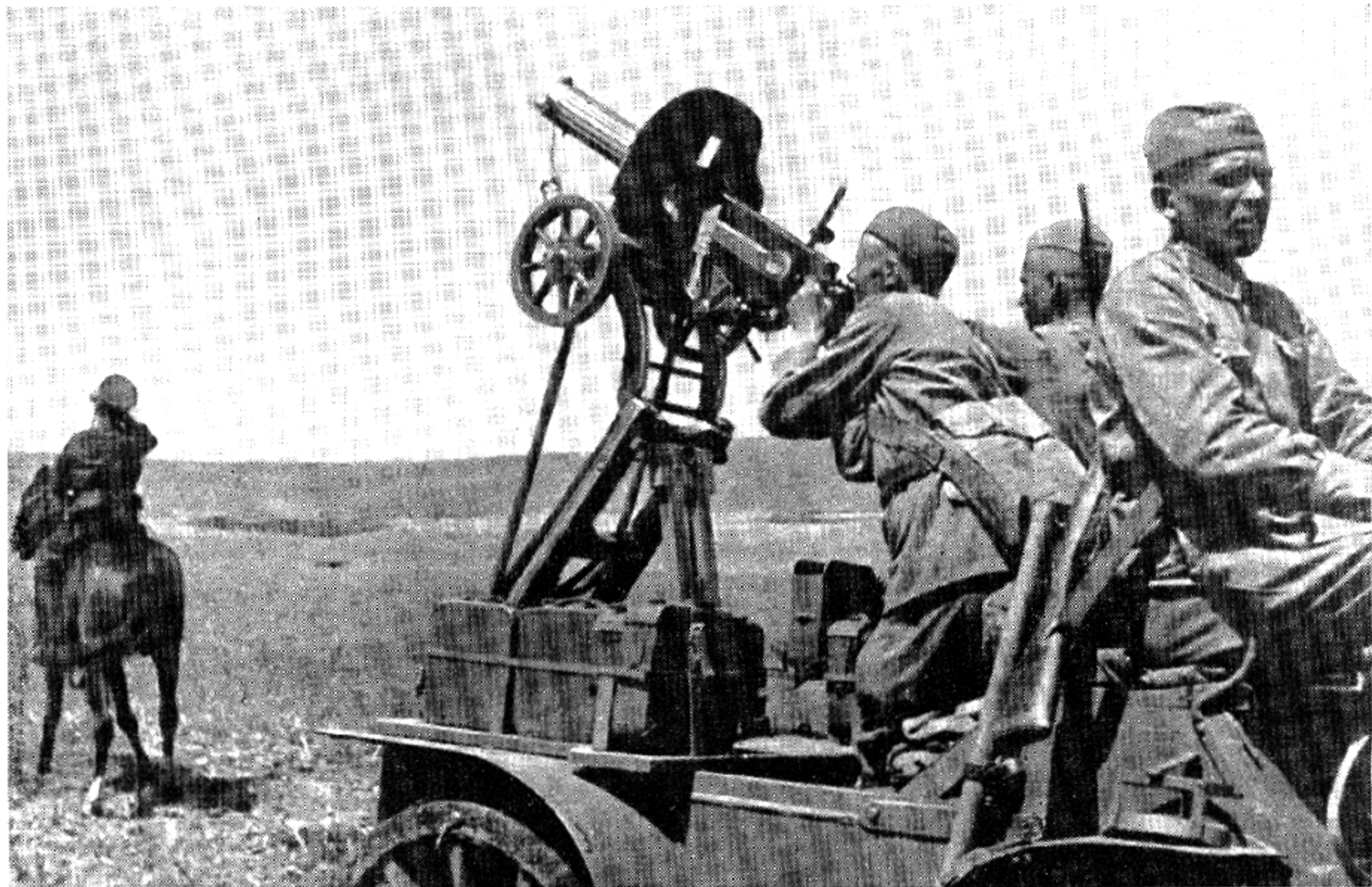
Figure 2-8. Soviet-Asiatic Troops in World War II with the Maxim Model 1910 on an AA Mount with horse-drawn transport.
