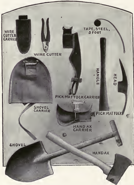
FIG. 3—UNITED STATES INFANTRY. TO EACH COMPANY OF 65 MEN: ONE 2-FOOT RULE, 21 SHOVELS WITH CARRIERS, 1 60-FOOT AND 1 5-FOOT STEEL TAPE, 3 HAND AXES AND CARRIERS, 7 PICK-MATTOCKS AND CARRIERS, AND 9 WIRE CUTTERS AND CARRIERS
