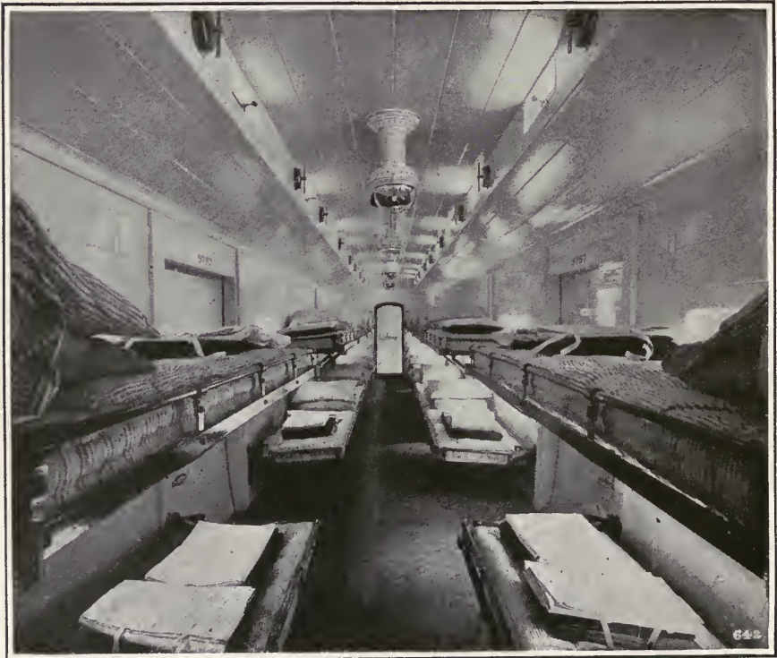
VIEW DOWN THE CENTER OF WARD CAR OF AN ENGLISH MILITARY AMBULANCE TRAIN, SHOWING FIXED BERTHS AND COTS. IN THE CENTER OF EACH TRAIN IS A PHARMACY CAR WITH TREATMENT ROOM, OFFICE, AND ALL NECESSARY SUPPLIES
