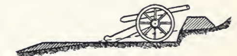
FIG. 24—SIMPLE GUN PIT ON CREST OF A HILL. GUN IN POSITION FOR DIRECT FIRING
