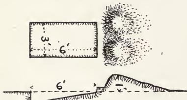
FIG. 9—LYING DOWN TRENCH
