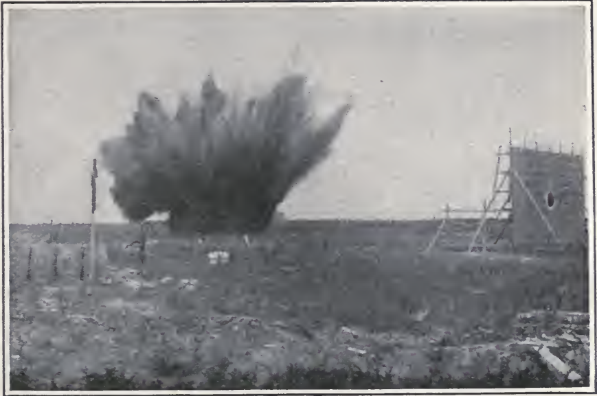
DETONATION OF A 12-INCH SHELL FILLED WITH HIGH EXPLOSIVE AND BURIED SIX FEET BELOW GROUND
