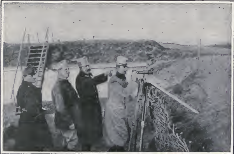
A FIELD TELEMETER OR RANGE-FINDER AS USED BY OFFICERS OF THE AUSTRIAN ARMY TO STUDY THE POSITIONS OF THE RUSSIAN FORCES. THE OBSERVERS, CONCEALED BEHIND BREASTWORKS, ARE ENDEAVORING TO LOCATE AND DETERMINE THE RANGE OF THE HIDDEN BATTERIES OF THE ENEMY IN ORDER TO DIRECT THE FIRE OF THEIR OWN GUNS
