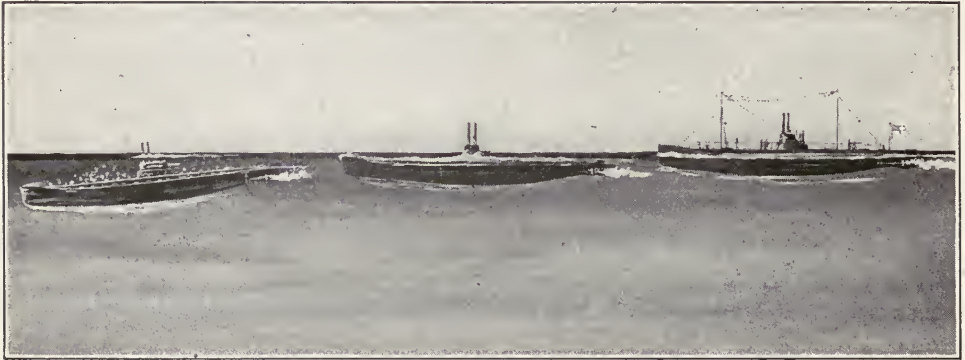
THREE POSITIONS OF THE SUBMARINE—DIVING, AWASH AND SURFACE NAVIGATION
