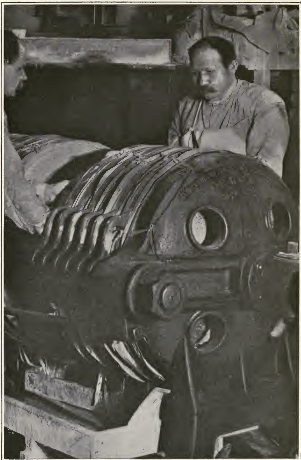
THE FILTER PRESS IS LARGELY USED IN THE MANUFACTURE OF EXPLOSIVES
