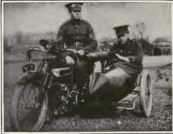
BRITISH SIDECAR FITTED WITH A LEWIS MACHINE GUN
