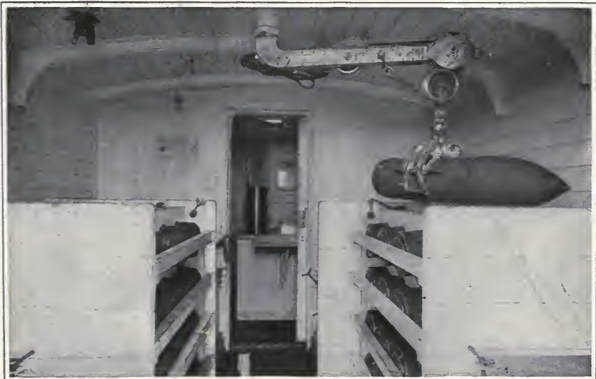
INTERIOR OF AMMUNITION CAR; CRANE PICKING UP SHELL FROM THE SHELL RACK
