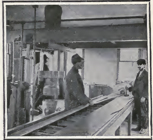
THE POWDER IS FORCED THROUGH MACARONI DIES IN THE FORM OF ENDLESS ROPE, PERFORATED FROM END TO END WITH A CONCENTRIC GROUP OF CIRCULAR PASSAGES
