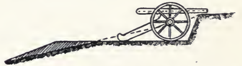
FIG. 23—SIMPLE GUN PIT. GUN IN POSITION FOR INDIRECT FIRING OVER THE CREST OF THE HILL
