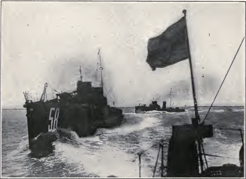
GROUP OF DESTROYERS MANEUVERING AT FULL SPEED. DATE, 1909. TONS, 650. SPEED, 32.5 KNOTS. GUNS, TWO 24-POUNDERS. TORPEDO TUBES, 3
