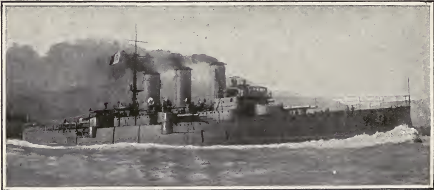
PRE-DREADNOUGHT "PISA." DISPLACEMENT, 11,000 TONS. SPEED, 22 KNOTS. GUNS, FOUR 10-INCH, EIGHT 7.5-INCH. BELT, 8-INCH
