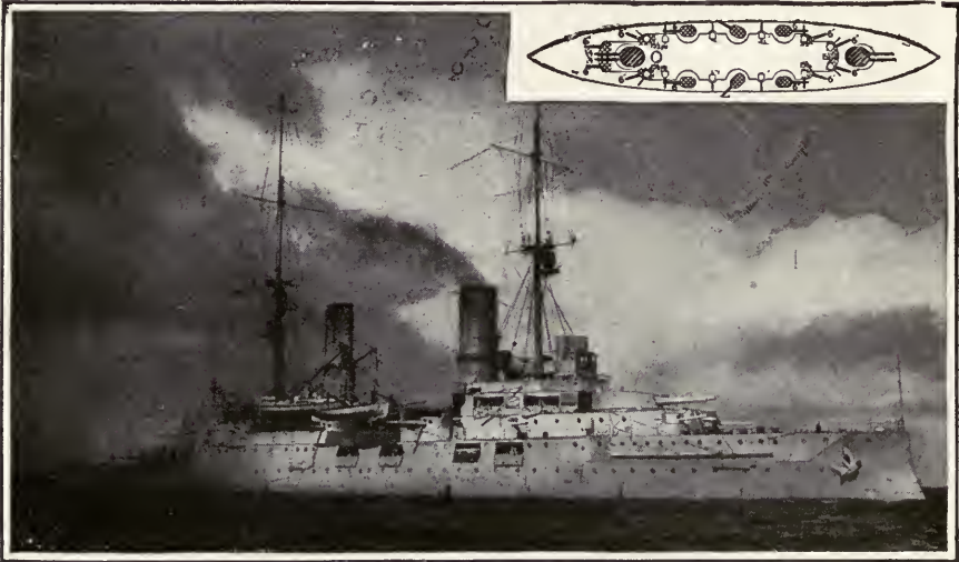
PRE-DREADNOUGHTS: "KAISER WILHELM II"; "KAISER FRIEDERICH III"; "KAISER BARBAROSSA"; "KAISER WILHELM DER GROSSE"; "KAISER KARL DER GROSSE." DATE, 1898-1901. TONS, 10,800. SPEED, 18 KNOTS. GUNS, FOUR 9.4-INCH, EIGHTEEN 6-INCH. TORPEDO TUBES, 6. SIDE ARMOR, 9-INCH—6-INCH
