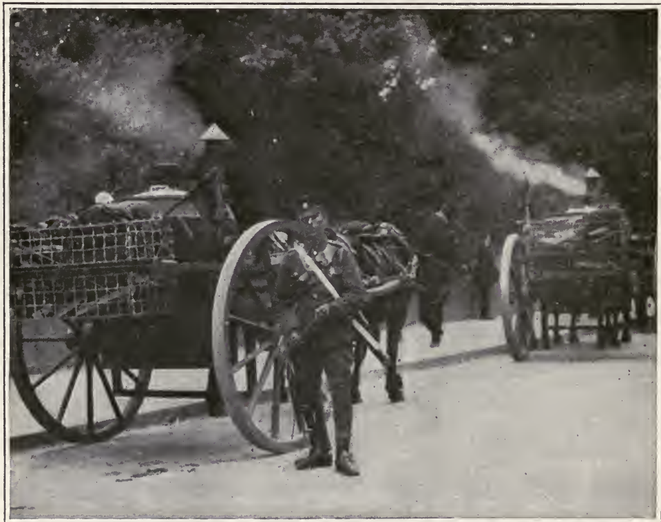
A NEW FORM OF FIELD OVEN USED BY THE BRITISH. THE MEAL IS COOKED BY THE TIME CAMP IS REACHED
