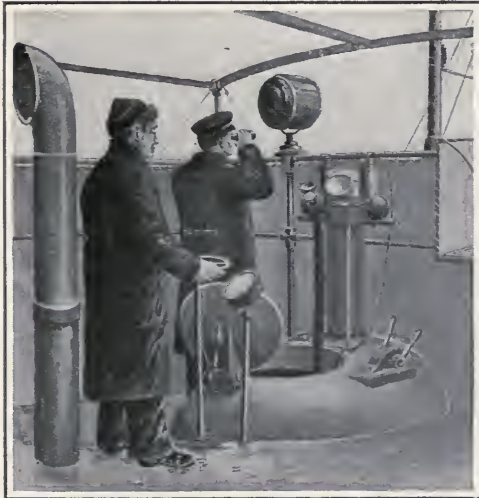
THE BRIDGE OF U.S.S. "G-2." AS FITTED FOR SURFACE CRUISING. THIS STRUCTURE IS MADE OF PORTABLE PARTS, FLOOR, STANCHIONS, RAILS, STEERING WHEEL, COMPASSES, CHART TABLE, SEARCHLIGHT AND VENTILATOR, ALL OF WHICH CAN BE REMOVED IN A SHORT TIME AND STOWED BELOW DECKS OR IN THE HOLLOW SUPERSTRUCTURE, LEAVING NOTHING BUT THE BARE CONNING TOWER
