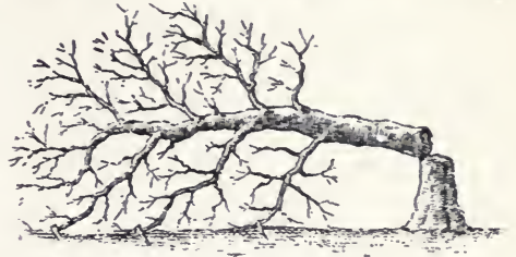
FIG. 31—FELLED TREE OBSTACLE. BRANCHES POINTING OUTWARD
