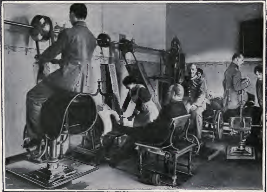
MOTOR-DRIVEN APPARATUS FOR MASSAGE OF FOOT AND BACK AND PERCUSSION OF ARMS; TO LEFT, CONVALESCENT ON RIDING APPARATUS
