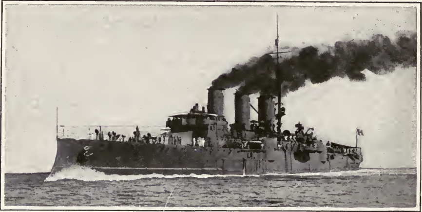
PRE-DREADNOUGHT "AMALFI." DISPLACEMENT, 11,000 TONS. SPEED, 23½ KNOTS. GUNS, FOUR 10 INCH, EIGHT 7.5-INCH. BELT, 8-INCH
