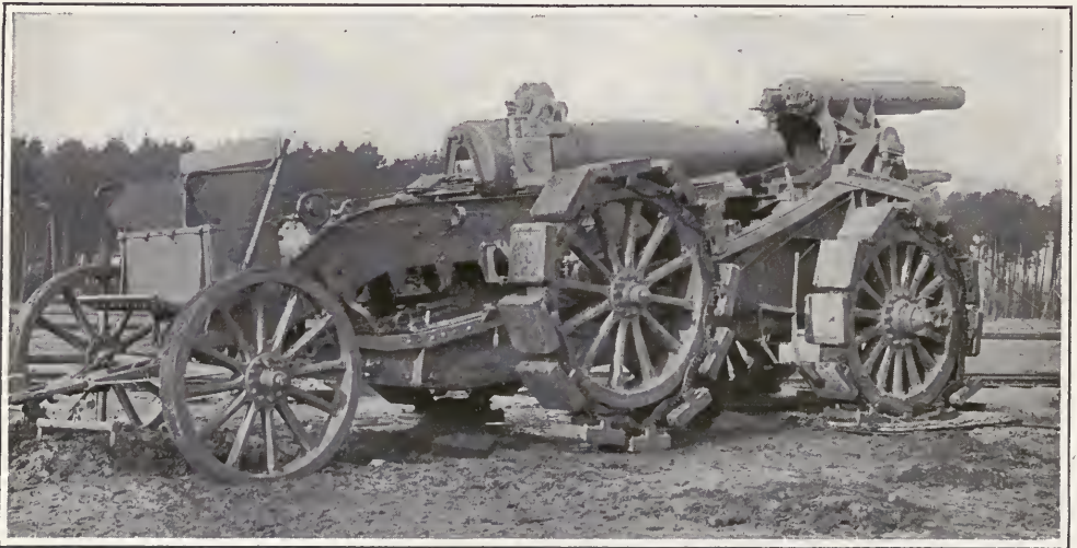
THE MORTAR BEING TRANSFERRED FROM ITS TRANSPORT CRADLE TO THE MOUNTING
