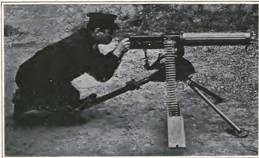
VICKERS AUTOMATIC RIFLE-CALIBER GUN ON ADJUSTABLE TRIPOD. SEAT BEING USED AS KNEE PAD
