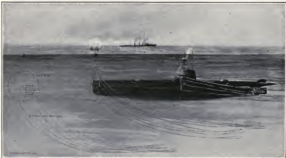
RENO PLAN OF CATCHING SUBMARINES BY TRAILING ROPES ATTACHED TO SUBMERGED RINGS, THE ROPES FOUL THE PROPELLERS. HER DISTRESS WILL BE NOTICED BY COSTON LIGHTS IGNITED AT THE SURFACE
