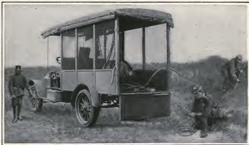
MOTOR TRUCK FITTED WITH AN ELECTRIC GENERATOR FOR FIELD USE
