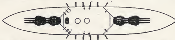
DREADNOUGHTS: "VIRIBUS UNITIS"; "TEGETTHOFF"; "SVENT ISTVAN." DATE, 1913-14. TONS, 20,000. SPEED, 20.7 KNOTS. GUNS, TWELVE 12-INCH. TORPEDO TUBES, 4. SIDE ARMOR, 11-INCH, 8-INCH, 6-INCH
