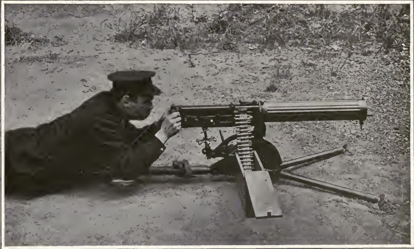
LOWEST FIRING POSITION WITH ADJUSTABLE TRIPOD. GUN 16 INCHES ABOVE GROUND. ANGLE ELEVATION DOES NOT ALTER IN TRAINING. SEAT BEING USED AS ELBOW REST
