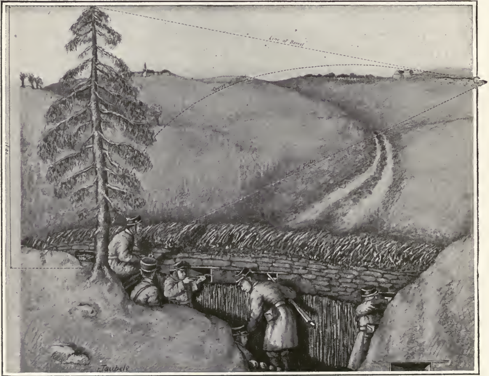
TO LAND IN THESE TRENCHES AT THE RANGE OF 1,000 YARDS, THE GERMAN MAUSER IS ACTUALLY POINTED AT THE TOP OF THE TREE, 40 FEET ABOVE THE GROUND, ALTHOUGH THE SIGHTS ARE ALIGNED ON THE TRENCHES. THE 0.450.70 SPRINGFIELD OF INDIAN FIGHTING DAYS WOULD HAVE TO BE POINTED 175 FEET ABOVE THE LINE OF TRENCHES TO REACH THEM.
