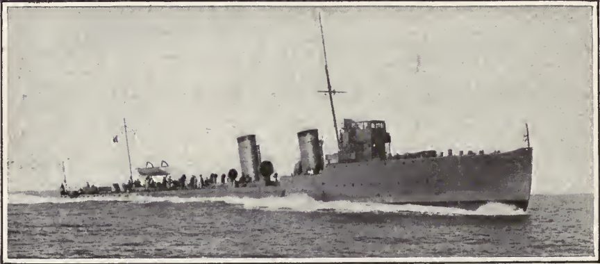
DESTROYER "AUDACE." DISPLACEMENT, 700 TONS. SPEED ON TRIAL, 36 KNOTS. GUNS, ONE 4.7-INCH, FOUR 3-INCH. TORPEDO TUBES, 2
