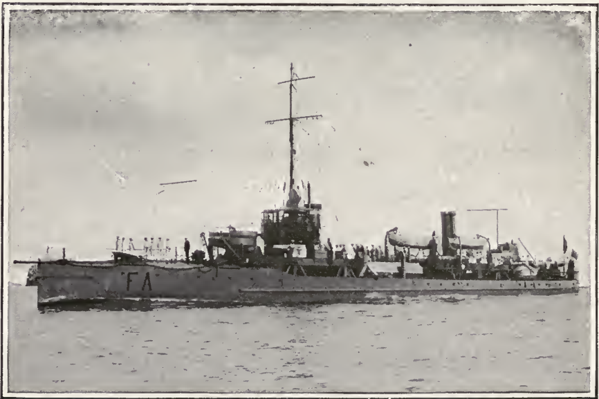
TORPEDO-BOAT DESTROYER: "FANION." DATE, 1908. TONS, 430. SPEED, 28 KNOTS. GUNS, ONE 9-POUNDER, SIX 3-POUNDERS. TORPEDO TUBES, 3
