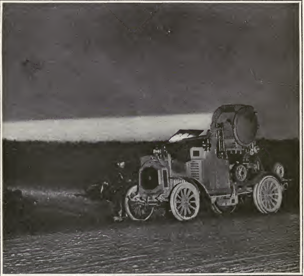
AUTOMOBILE-MOUNTED SEARCHLIGHT IN USE BY THE FRENCH ARMY
