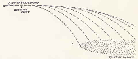
FIG. 8—THE GROUND COVERED BY A SHRAPNEL IS ELLIPTICAL IN FORM AND AT THE EFFECTIVE RANGES DOES NOT EXCEED 200 YARDS IN DEPTH BY 25 IN WIDTH. SHRAPNEL IS THE MOST IMPORTANT PROJECTILE. THE CASE IS OF DRAWN STEEL WITH SOLID BASE. THE MOUTH OF THE CASE HAS AN ALUMINIUM HEAD SCREWED IN AND TAPPED TO TAKE A COMBINATION TIME AND PERCUSSION FUSE. THE CASE CONTAINS 262 BALLS, EACH 0.49 INCH IN DIAMETER. THE BURSTING CHARGE CONSISTS OF 2 3-4 OUNCES OF LOOSE BLACK POWDER; IT IS PLACED IN THE BASE, AND COVERED BY A STEEL DIAPHRAGM. THE FUSE IS TIMED SO THAT THE CASE WILL BURST JUST IN FRONT AND ABOVE THE TRENCHES OR LINE OF TROOPS.
