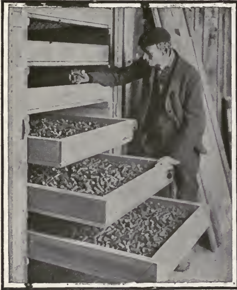
IN THE DRYING HOUSE, WHERE THE POWDER GRAINS ARE STORED AWAY AND DRIED TO THE PROPER STAGE, BEFORE TESTING AND SEALING AWAY IN AIR-TIGHT TANKS
