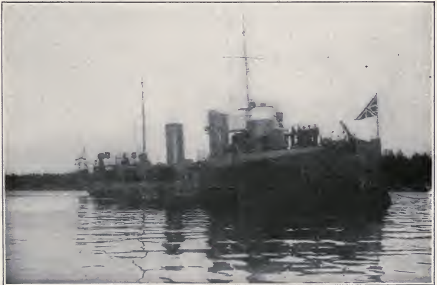
TORPEDO-BOAT DESTROYERS: "KONDRATENKO"; "OKHOTNIK"; "POGRANITSCHNIK"; "SIBERSKIJ-STRELOK." DATE, 1905. TONS, 625. SPEED, 26 KNOTS. GUNS, TWO 3-INCH, SIX 6-POUNDERS. TORPEDO TUBES, 3
