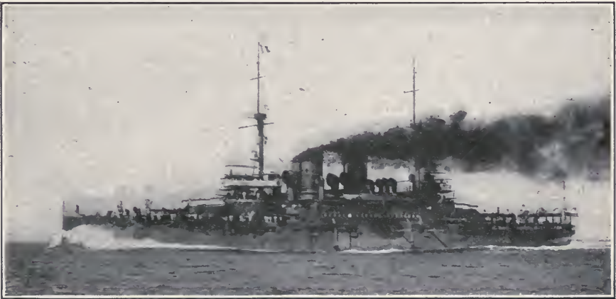
PRE-DREADNOUGHT "BENEDETTO BRIN." DISPLACEMENT, 13,500 TONS. SPEED, 20 KNOTS. GUNS, FOUR 12-INCH, FOUR 8-INCH, TWELVE 6-INCH. BELT, 6-INCH
