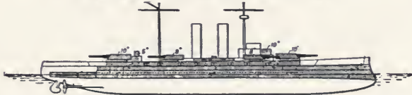
DREADNOUGHTS: "VIRIBUS UNITIS"; "TEGETTHOFF"; "SVENT ISTVAN." DATE, 1913-14. TONS, 20,000. SPEED, 20.7 KNOTS. GUNS, TWELVE 12-INCH. TORPEDO TUBES, 4. SIDE ARMOR, 11-INCH, 8-INCH, 6-INCH
