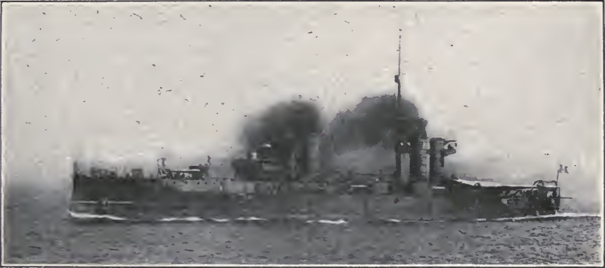
PRE-DREADNOUGHT "SAN MARCO." DISPLACEMENT, 10,000 TONS. SPEED, 24 KNOTS. GUNS, FOUR 10-INCH, EIGHT 7.5-INCH. BELT, 8-INCH
