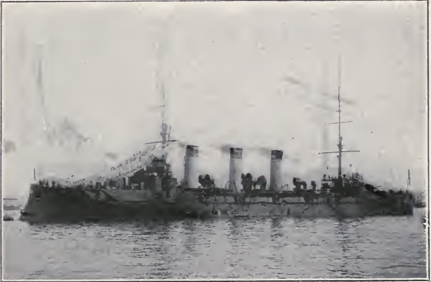
PROTECTED CRUISERS: "OLEJ"; "BOGATYR." DATE, 1902-04. TONS, 6,675. SPEED, 23-24 KNOTS. GUNS, TWELVE 6-INCH, TWELVE 3-INCH. TORPEDO TUBES, 4. ARMOR, 3-INCH DECK
