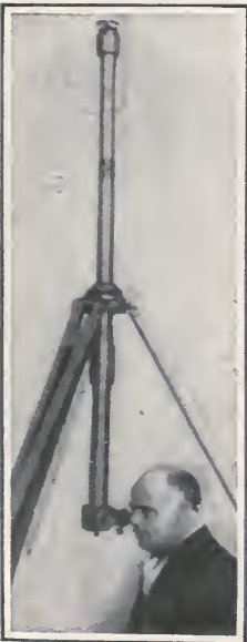
THE WHOLE HORIZON IS VISIBLE WITH PANORAMIC PERISCOPE
