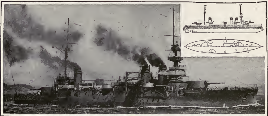
PRE-DREADNOUGHTS: "JUSTICE"; "DEMOCRATIC"; "VERITE." DATE, 1907-1908. TONS, 14,900. SPEED, 19.4 KNOTS. GUNS, FOUR 12-INCH, TEN 7.6-INCH. TORPEDO TUBES, 4. SIDE ARMOR, 11-INCH.
