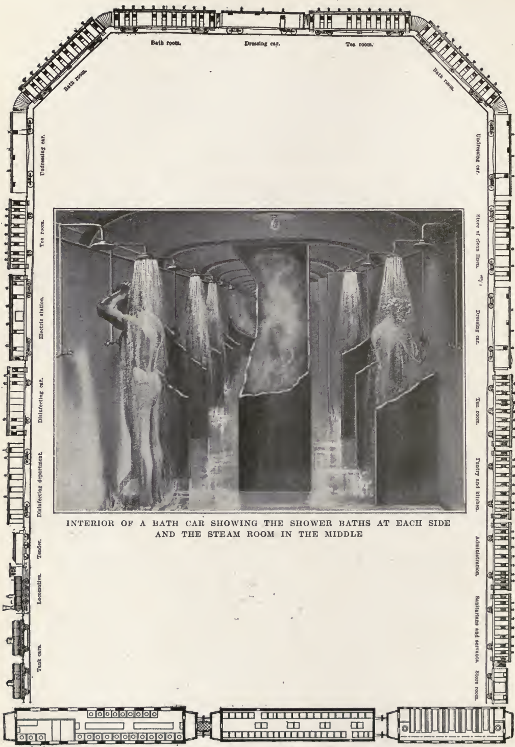
SECTIONAL PLAN VIEW OF THREE CARS OF A RUSSIAN ARMY BATH TRAIN
