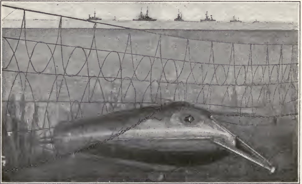
PASSING BELOW PROTECTIVE NETTING. WHEN THE SUBMARINE, TRAVELING ON THE BOTTOM, REACHES THE NET, THE LATTER IS LIFTED BY THE PROJECTING ARMS AND SLIDES OVER THE SMOOTH BODY OF THE BOAT
