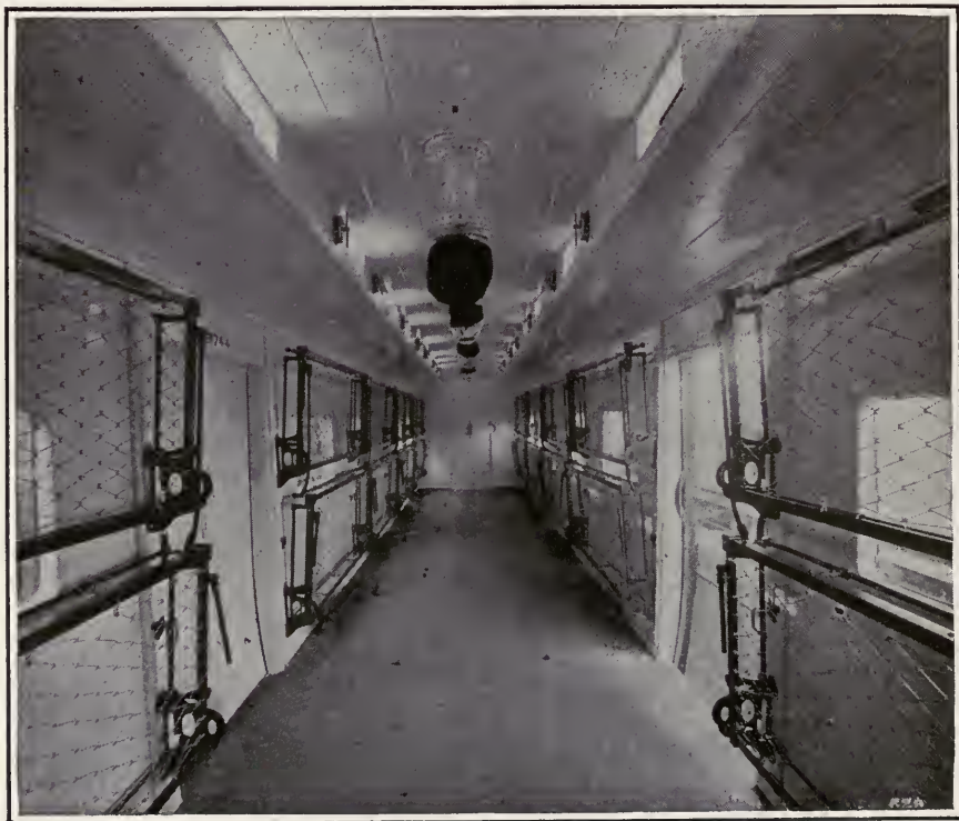
THE WARD CARS OF THE BRITISH AMBULANCE TRAINS WERE CONVERTED FROM OPEN FREIGHT CARS. THEY WERE REFLOORED, AND HOOKS WERE FIXED IN THE CEILINGS FOR SUSPENDING FOLDING COTS IN TWO TIERS ON BOTH SIDES
