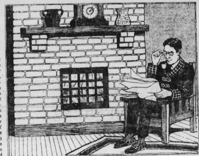
The Front of the Ground Floor Furnace Is in the Living Room. The Glowing Coals Can Be Seen Through the Mica Windows Which Produce the Effect of an Open Fireplace.
